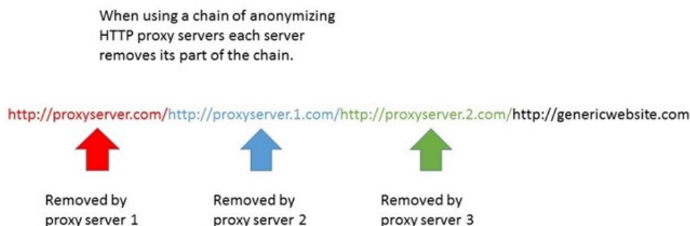
Figure 3. Rewebber chain constructed using three rewebbers
