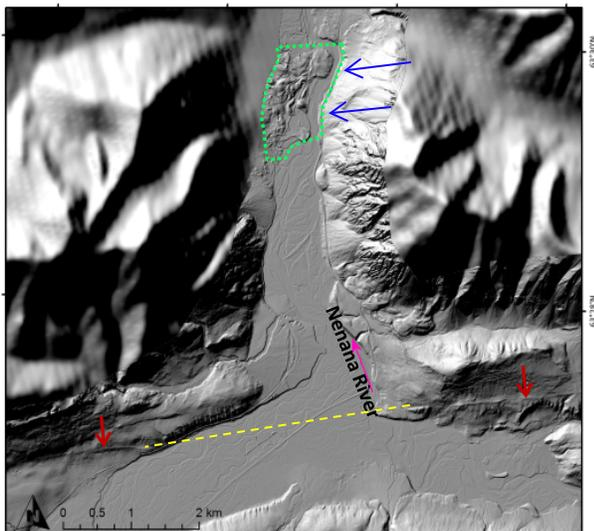
**Figure 1:** Shaded relief topographic map of the study area: red – visible fault scarp; yellow – projected fault trajectory; green – outline of landslide deposit; blue – landslide source and direction of flow; pink – river flow direction.
