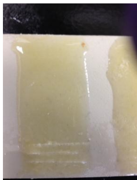
Figure 9—Polyurethane films; without microcapsules (left) and with microcapsules (right).
