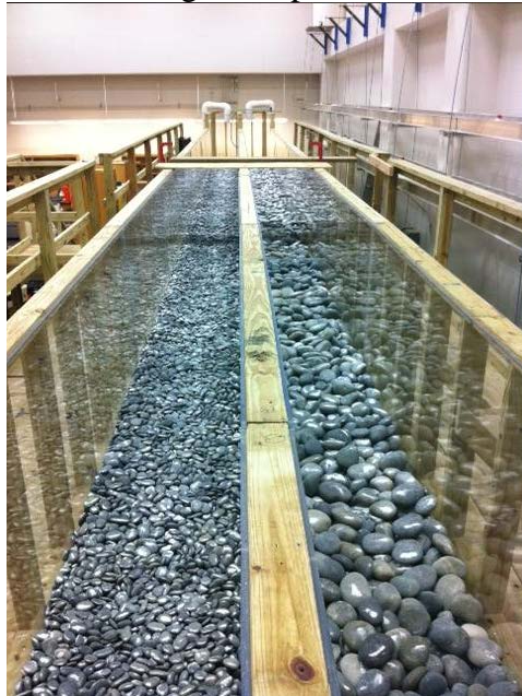
photograph of 2 flumes running parallel to each other, the flume on the right contains the cobbles and the flume on the left contains the gravels
