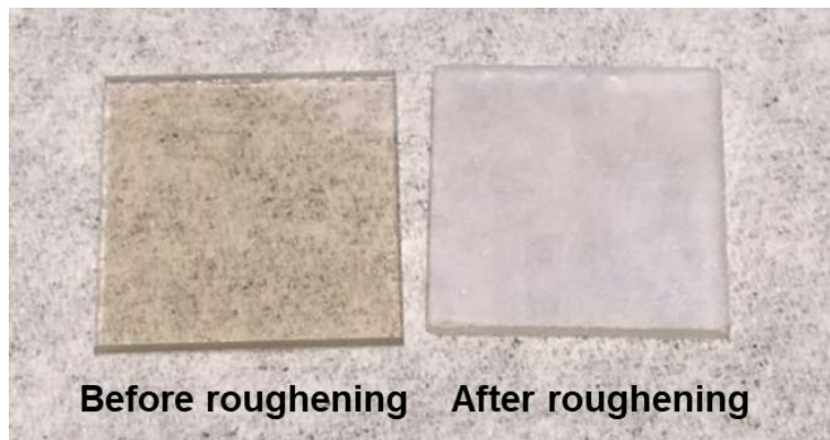
Figure S1. A photograph of ITO thin films grown on glass substrates. As-grown ITO thin films are transparent because of the high transparency of the ITO thin film and the glass substrate (left). For the optical spectroscopic ellipsometry measurements, we have prepared samples by roughening the backside of the substrates using sandpaper (right).
