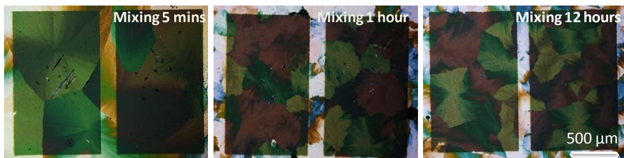
Figure S1. Polarized optical micrographs of the channel regions of TES-ADT FETs with different grain boundaries.
