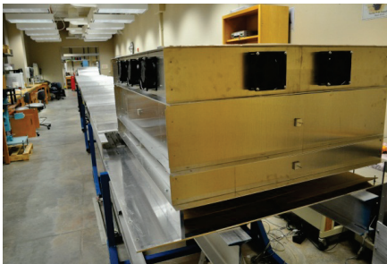
Figure 1: Blowing rig in place on test section of turbulent channel flow facility.
