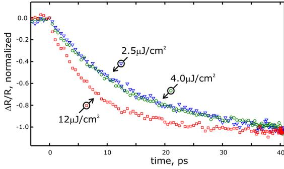
FIG. 1: **Pump-probe spectroscopy at 5K** Pump pulse ( $1.5\text{eV}$ ) fluence dependence of the transient response of  $\text{Na}_2\text{IrO}_3$ . The decay rate of normalized curves is fluence independent for low fluence values indicating that in this regime the magnetic order is not melted by the pump pulse.
