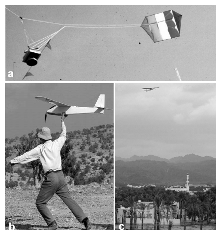
Figure 1 Kite (a) and remotely controlled drone (b and c) taking true colour and near-infrared aerial images of grass and bush vegetation.
