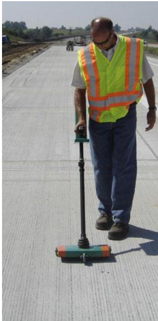
Figure 3 MIT-T2 Scanning Device (Courtesy J. Gudimettla TRB 2019)
