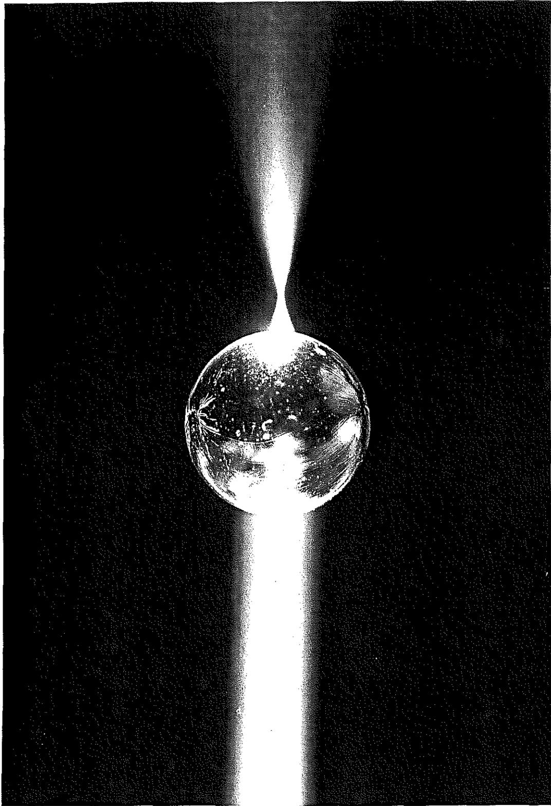
Photograph showing the convergence of a beam of light by refraction at the surface of a glass sphere. This is a practical illustration of an otherwise theoretical analysis of the optical properties of sign surfaces.
