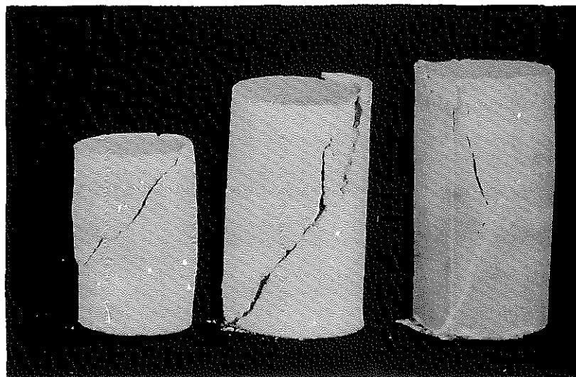
Untreated Thermally Treated Thermally Treated to 600°C. to 850°C
