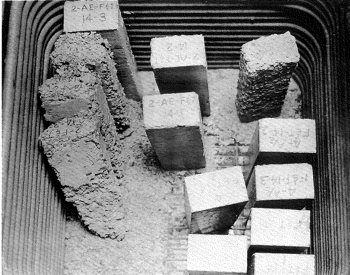
Fig. 3: Photograph Showing DGA Concrete Specimens in F & T Chamber after about 25 Cycles. Specimens marked 2- and 4-AE are air-entrained concretes containing 2 and 4 bags of Type I cement, respectively. Deteriorated specimens are non-air concretes containing 2 and 3 bags of cement. Note: 2 specimens of non-air concretes containing 4 bags of cement per cu. yd. (center and lower right) remained in relatively good condition at this stage in the testing.
