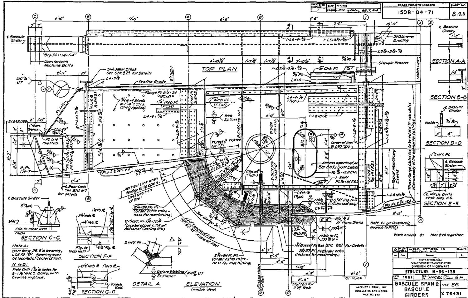
Figure 1. WisDOT Bascule Bridge Girder - Weldment Shown in Shaded Area.
