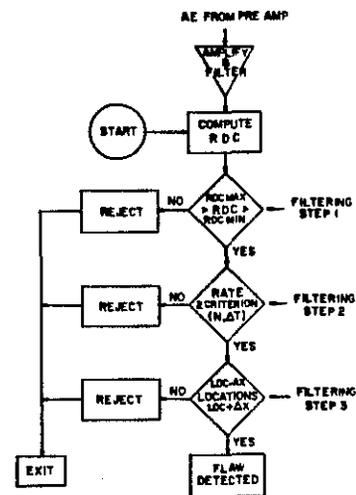
Figure 1. AEWM Processing Flow Chart for Flaw Detection.
