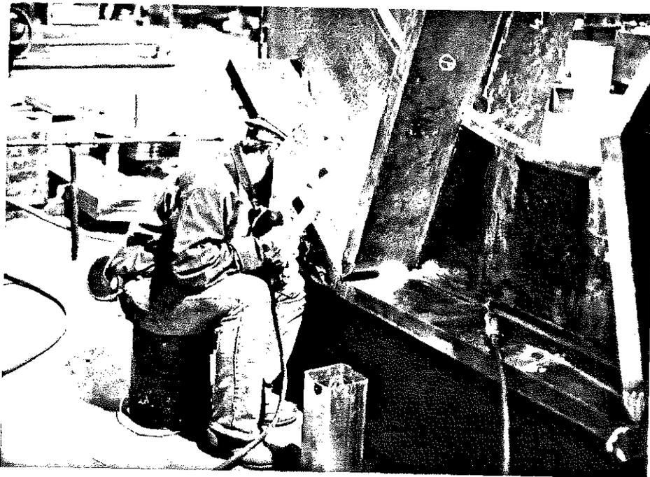
Figure 5. Depositing Full-Penetration Stiffener-to-Flange Welds Using Manual SMAW.
