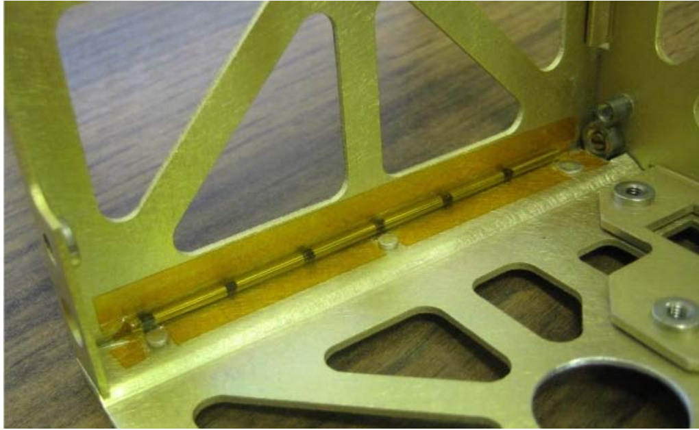
Figure 5-3: One of Four Alinco-5 Permanent Magnet sets on board KySat-1.
