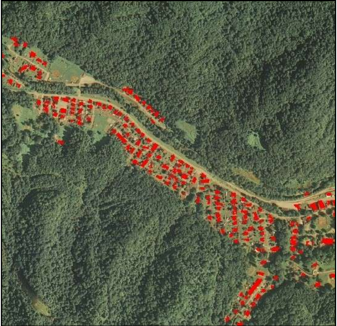
Figure 3.2. Buildings in southeastern Kentucky extracted from orthoimagery into a polygon shapefile using Feature Analyst 4.2 (Visual Learning Systems, Missoula, MT) and used in the black bear study 2005-08.
