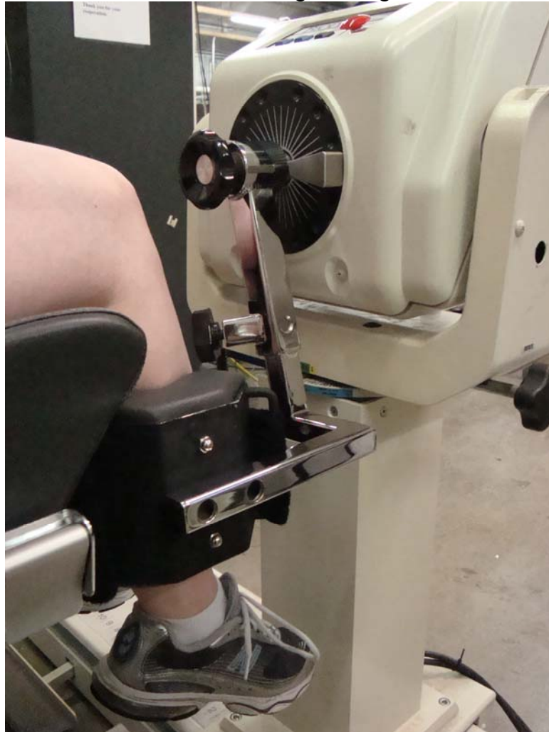
Figure 3.2: Setup of subject on Biodex for internal and external rotation strength testing
