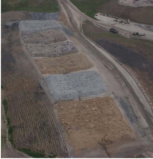
FIGURE 2.1. Aerial view of the 2005 loose-dumped plots at the Bent Mountain surface mine in Pike County, Kentucky. The size of each plot is approximately 0.4-hectare.
