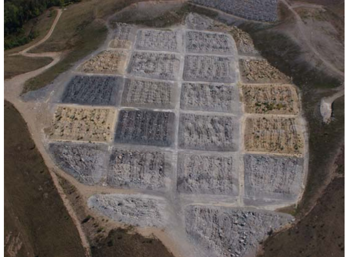
FIGURE 2.2. Aerial view of the 2007 loose-dumped plots. The size of each plot is approximately 0.2-hectare.
