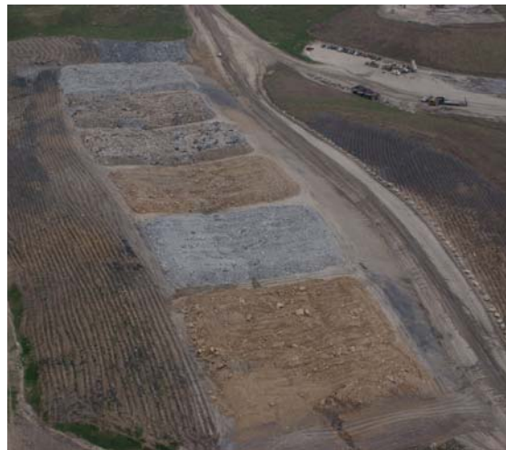
FIGURE 1.2. Aerial view of the 2005 loose-dumped plots at the Bent Mountain surface mine in Pike County, Kentucky. The size of each plot is approximately 0.4 hectare.
