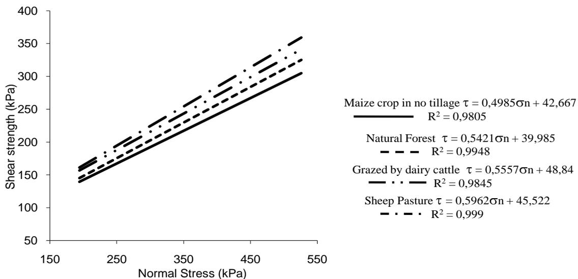
Figure 2. Shear rupture lines of an LVAd submitted to different managements, with samples at a water tension of -6 kPa.
