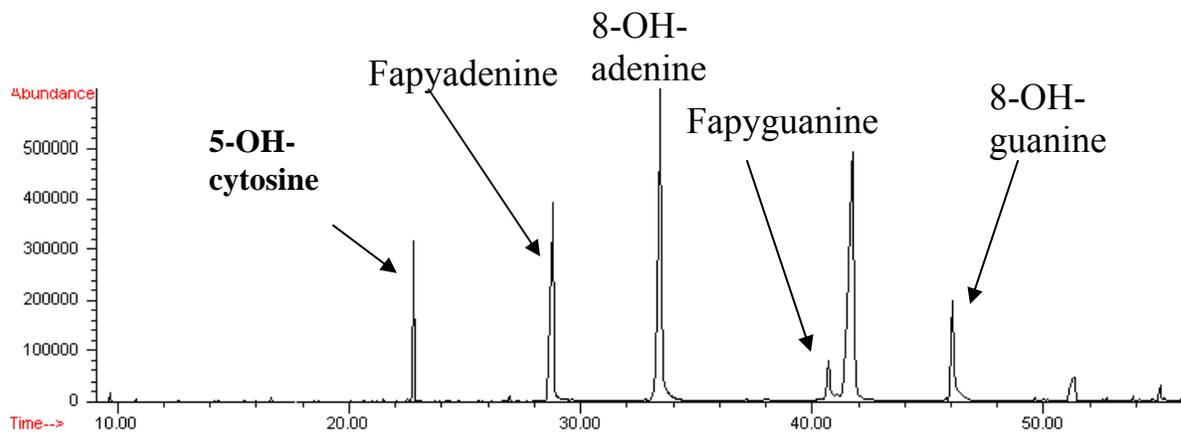
**Figure 2.2.** Representative chromatogram of DNA oxidized adducts.
