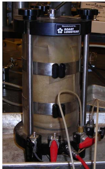
Figure 5.1. Sample setup showing triaxial cell and sample close-up.
