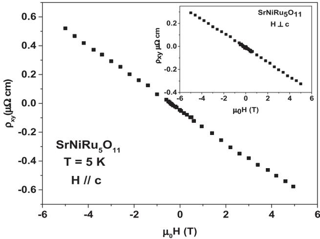
FIG. 7. Transverse resistivity  $\rho_{xy}$  versus magnetic field  $\mathbf{H} \parallel \mathbf{c}$  axis for single-crystal  $\text{SrNiRu}_5\text{O}_{11}$  at temperature  $T = 5$  K. Inset: The transverse resistivity  $\rho_{xy}$  versus magnetic field  $\mathbf{H} \perp \mathbf{c}$  axis for single-crystal  $\text{SrNiRu}_5\text{O}_{11}$  at  $T = 5$  K.
