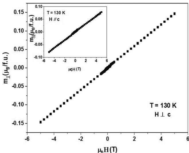
FIG. 6. Magnetic moment for applied field  $H$  perpendicular to the  $c$  axis,  $m_{\perp}$ , versus  $H$  at temperature  $T = 130$  K. Inset: The moment for  $H$  perpendicular to the  $c$  axis,  $m_{\parallel}$ , versus  $H$  at  $T = 130$  K.
