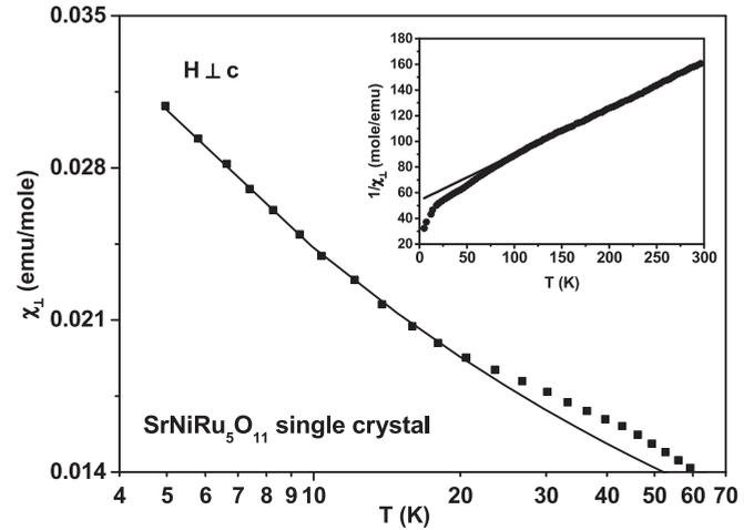
FIG. 3. Low-temperature magnetic susceptibility for field  $\mu_0 H = 0.5$  T applied perpendicular to the  $c$  axis,  $\chi_{\perp}$ , versus temperature  $T$ . The solid curve is a fit to  $\chi_{\perp} \sim T^{-0.3}$ . Inset: The inverse magnetic susceptibility  $(\chi_{\perp})^{-1}$  versus  $T$ ; the solid curve is a fit of the data to the Curie-Weiss law (see text for details).
