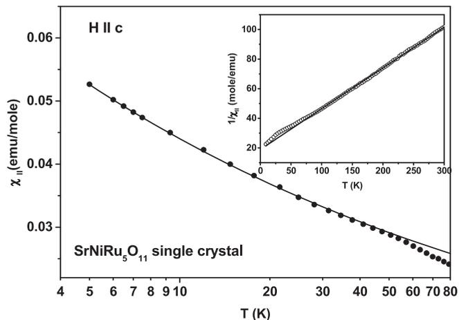
FIG. 4. Low-temperature magnetic susceptibility for magnetic field  $\mu_0 H = 0.5$  T applied parallel to the  $c$  axis,  $\chi_{\parallel}$ , versus temperature  $T$ . The solid curve is a fit to  $\chi_{\parallel} \sim T^{-0.3}$ . Inset: The inverse magnetic susceptibility  $(\chi_{\parallel})^{-1}$  versus  $T$ ; the solid curve is a fit of the data to the Curie-Weiss law (see text for details).
