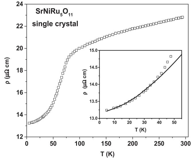
FIG. 8. Temperature dependence of the longitudinal electrical resistivity  $\rho = \rho_{xx}$  of single-crystal  $\text{SrNiRu}_5\text{O}_{11}$  with in-plane current  $\mathbf{J} \perp \mathbf{c}$  axis. Inset: The low-temperature resistivity, where the solid curve is a fit of the data to  $\rho_{xx} \sim T^{1.6}$ .
