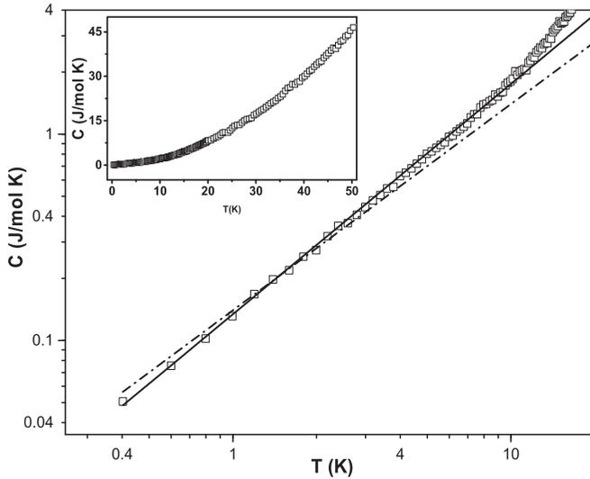
FIG. 9. Low-temperature specific heat  $C(T)$  of single-crystal  $\text{SrNiRu}_5\text{O}_{11}$  versus temperature  $T$  (note logarithmic scale). The dashed line is a fit of the data to Eq. (2) with power-law exponent  $\alpha = 1.0$ . The solid line is an improved fit using Eq. (2) with a modified electronic contribution,  $C_{el} = \gamma T^{1.2}$ . The inset shows the total specific heat  $C(T)$  data for single-crystal  $\text{SrNiRu}_5\text{O}_{11}$  over the temperature range 0.35–50 K.
