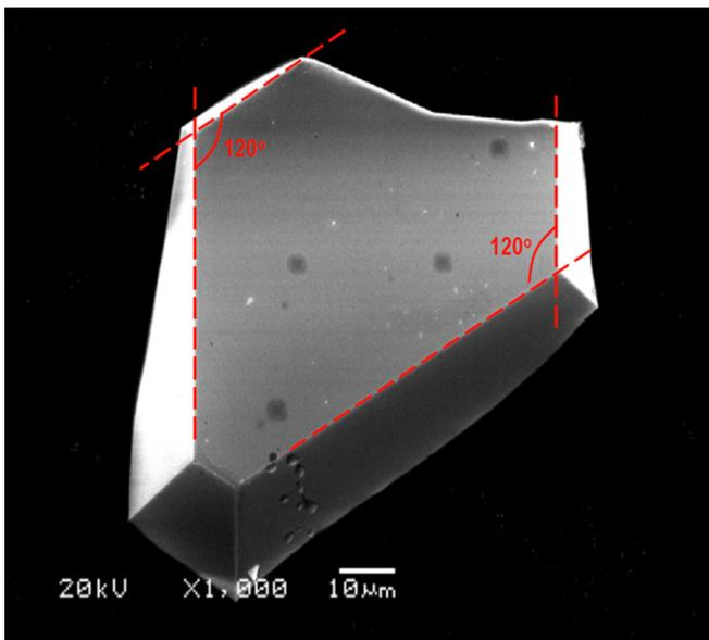
FIG. 2. Scanning electron microscopy image of a small crystal of  $\text{SrNiRu}_5\text{O}_{11}$ , revealing a hexagonal crystal habit, as shown by the characteristic angles highlighted by red dashed lines.
