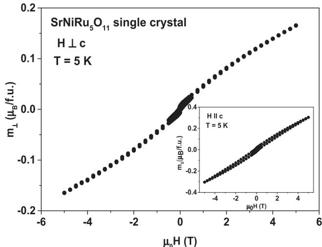
FIG. 5. Magnetic moment  $m_{\perp}$  perpendicular to the  $c$  axis versus magnetic field  $H$  at temperature  $T = 5$  K. Inset: The magnetic moment  $m_{\parallel}$  along the  $c$  axis versus magnetic field at  $T = 5$  K.
