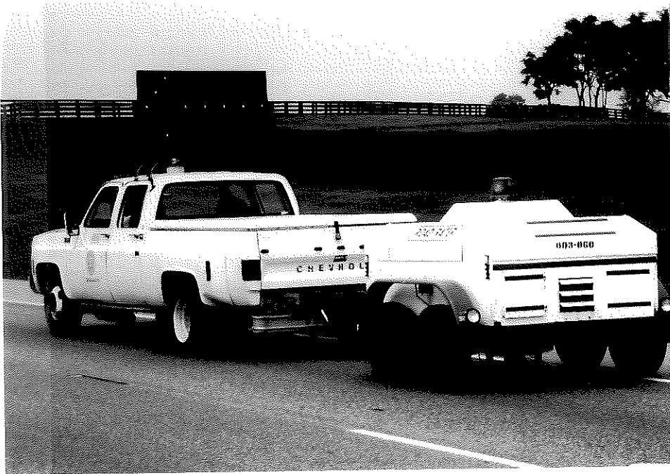
Figure 2. Kentucky Transportation Cabinet Model 2000 Road Rater
