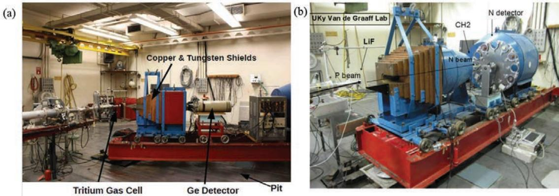
Fig. 2. The apparatus shown in Fig. 2(a) is used for most nuclear structure studies at UKAL, which utilizes primarily the  ${}^3\text{H}(p,n){}^3\text{He}$  reaction for neutron production. The setup shown in Fig. 2(b) is used for neutron transmission studies, with neutrons produced using the  ${}^3\text{Li}(p,n){}^3\text{He}$  reaction. Various targets are rotated into the beamline for the transmission studies by remote control.
