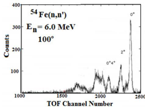
Fig. 8: Time-of-flight spectrum from  $^{54}\text{Fe}$  neutron scattering measurements. The elastic scattering peak is rightmost in the spectrum as time increases from right to left. The lowest levels are clearly observed, but above the first few levels, the individual states cannot be resolved.
