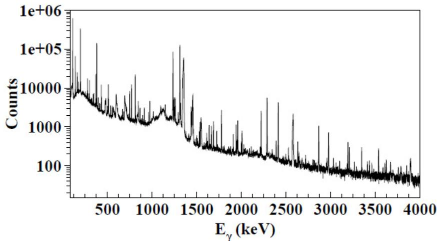
Fig. 7: Summed  $(n,n'\gamma)$  excitation function spectrum for  $^{136}\text{Xe}$  for incident neutron energies from 2.5 to 4.5 MeV in 0.25 MeV increments using a solid  $^{136}\text{XeF}_2$  scattering sample.
