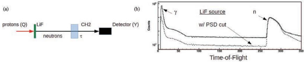
Fig. 4 (a) A schematic representation of the experimental configuration for measuring the  $n$ - $p$  total cross sections and (b) an experimental TOF spectrum, with and without PSD, for the neutron transmission measurements.
