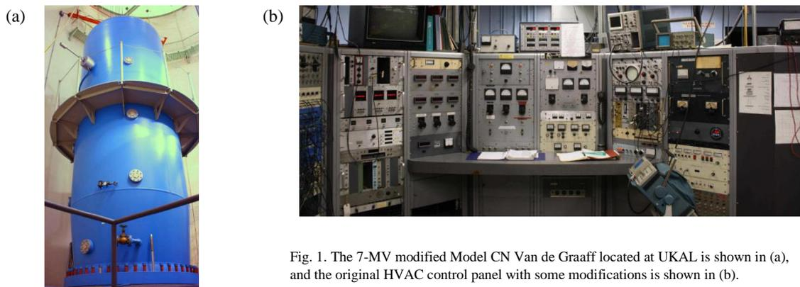
Fig. 1. The 7-MV modified Model CN Van de Graaff located at UKAL is shown in (a), and the original HVAC control panel with some modifications is shown in (b).
