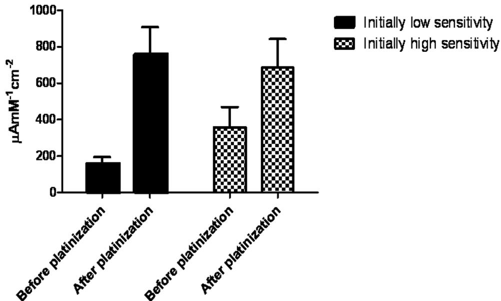
Figure 4.15: Effect of platinization on electrodes with different initial performance.
