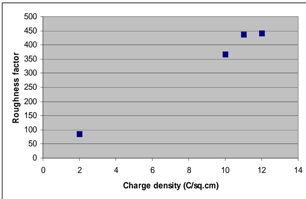
**Figure 4.7: Effect of charge density on the roughness factor of electrode surface.**
