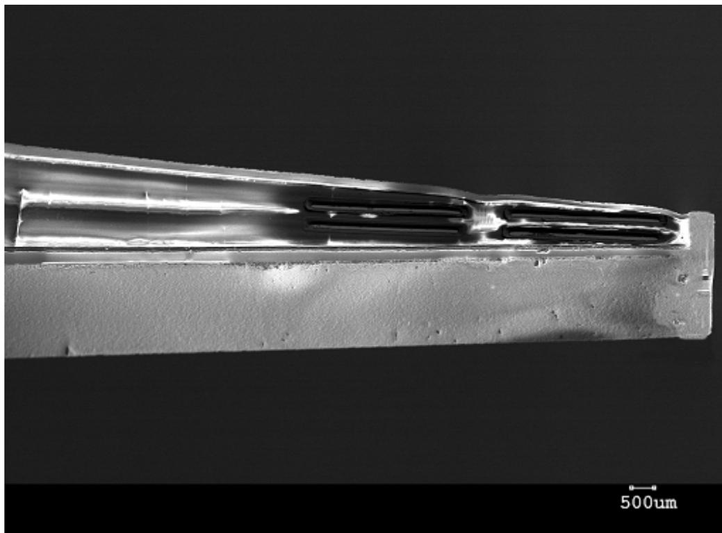
**Figure 4.5: SEM image of microelectrode tip tilted by 60°. Variations in signal level are the result of charging of the ceramic substrate and polyimide coating.**
