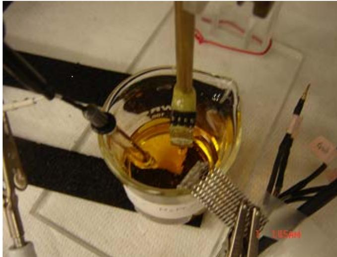
**Figure 3.2: Photograph of Platinum-black deposition on Platinum recording sites.**
