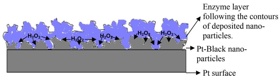
**Figure 4.16(b): Schematic diagram of thin enzyme layer covering the contours of rough Pt-Black surface. Most of the peroxide produced by L-glutamate decomposition is captured by rough electrode surface.**
