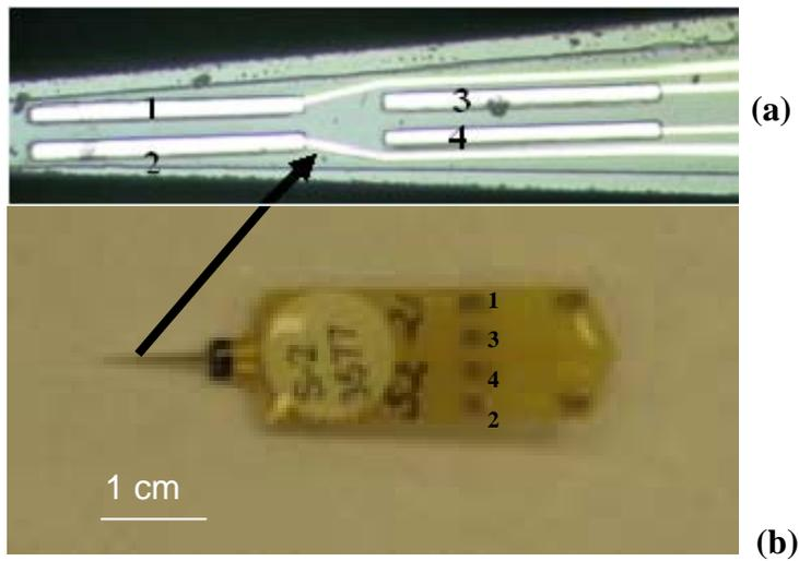
**Figure 1.1: Photograph of (a) 1 cm long ceramic based multisite microelectrode tip (b) multisite microelectrode bonded to a printed circuit board.**
