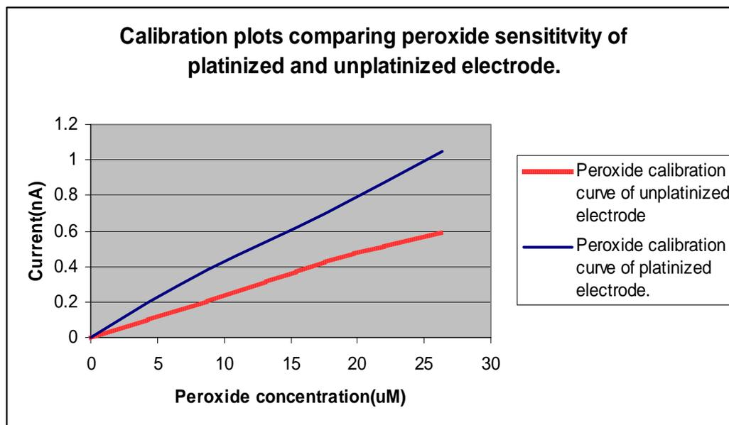
**Figure 4.14: Calibration curves for bare platinum electrode and Pt-Black deposited electrode.**
