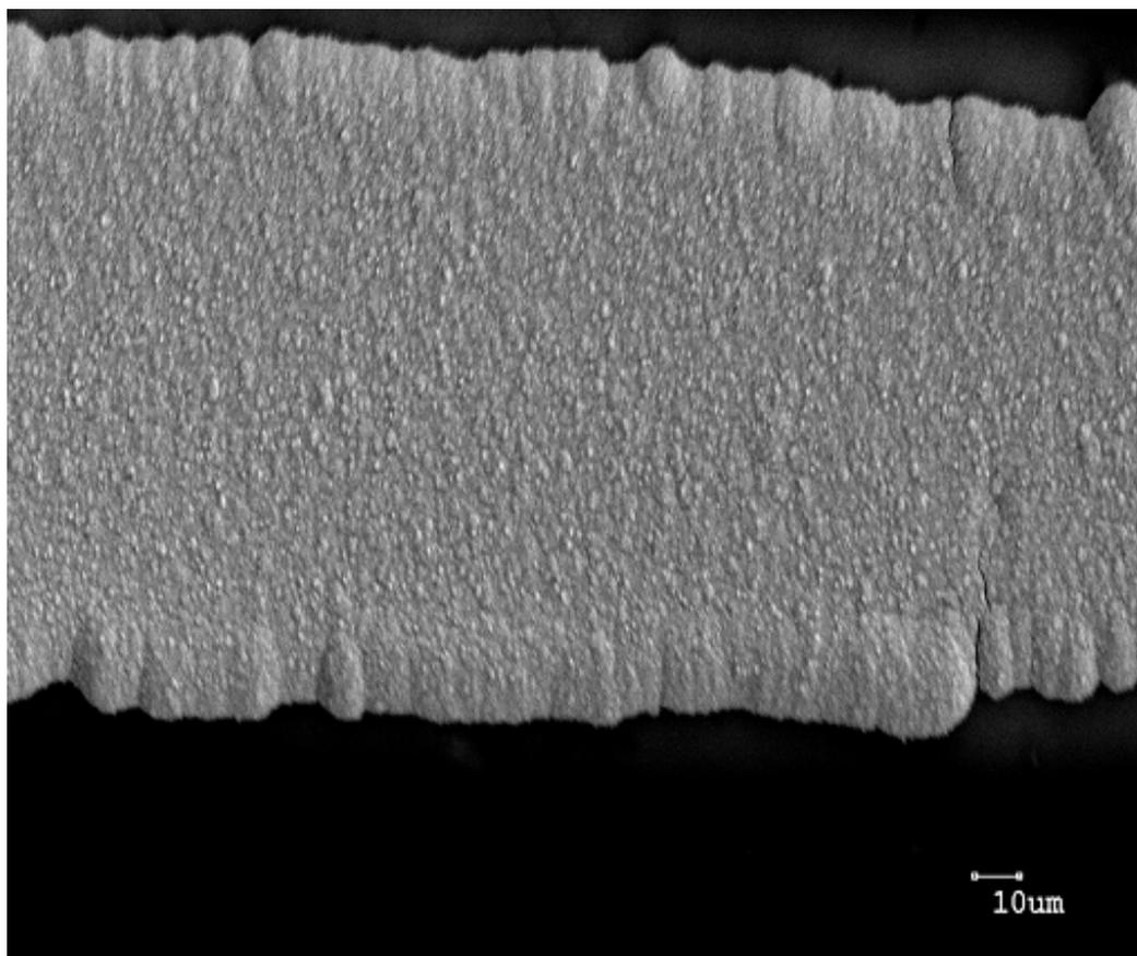
**Figure 4.4: SEM image of nanostructured platinum deposited at -0.12V Vs Ag|AgCl reference, deposition temperature was 25°C, and deposition charge density was 2Ccm<sup>-2</sup>.**
