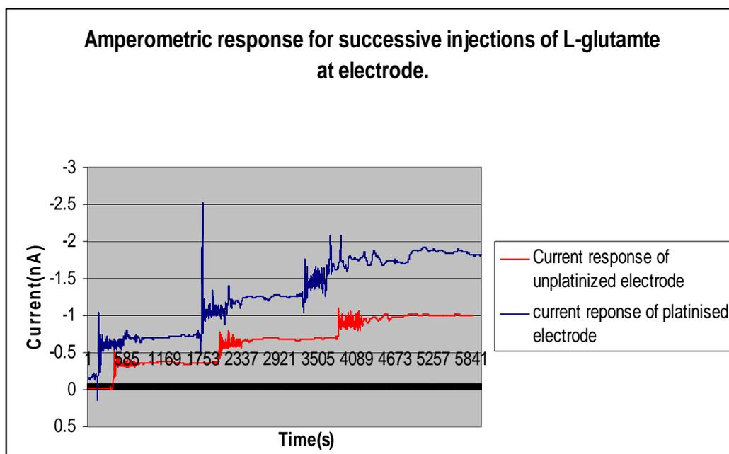
**Figure 4.17: Amperometric response for successive injections of glutamate at electrode surface. Applied potential was 700 mV vs Ag/AgCl reference. Cell volume: 40 mL. Injection volume 40  $\mu$ L of 20 mM of H<sub>2</sub>O<sub>2</sub>.**
