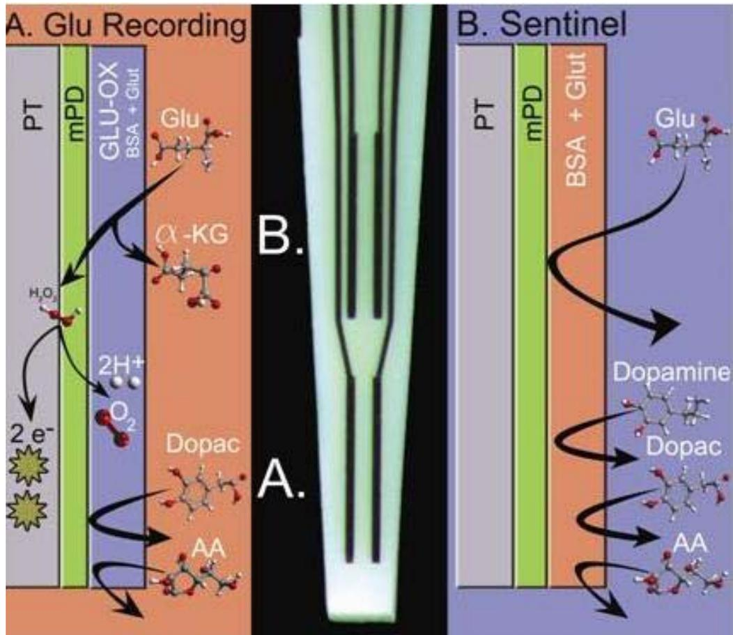
**Figure 2.3. Schematic drawing of the different layers present on the microsensor in order to measure glutamate (A). Recording sites with GluOx (B). Sentinel sites without GluOx.**
