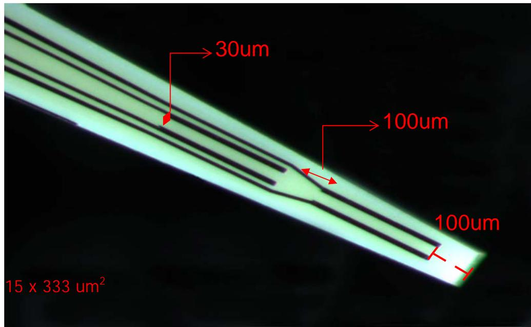
**Figure 2.2. Photograph of Pt multisite microelectrode. The recording sites are 15 μm wide by 333 μm long.**
