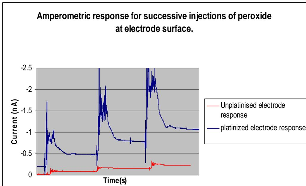
**Figure 4.13: Amperometric response for successive injections of  $H_2O_2$  at electrode surface. Applied potential was 700mV vs Ag/AgCl reference. Cell volume: 40mL. Injection volume: 40uL of 8.8mM of  $H_2O_2$ .**
