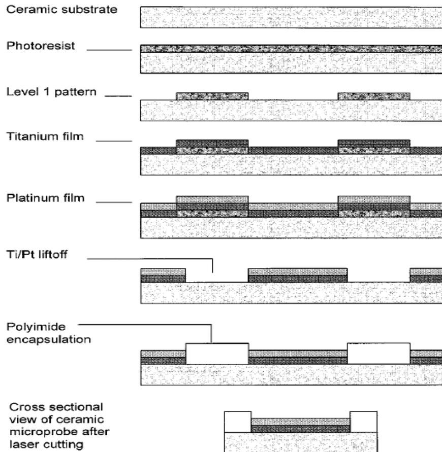
**Figure 2.1. Schematic diagram illustrating the fabrication steps of the ceramic-based multisite microelectrodes. Reproduced from [12]**
