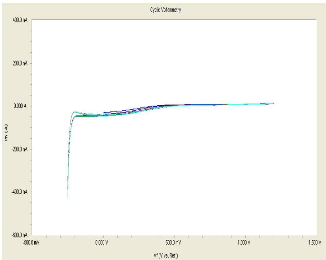
**Figure 4.8:** Cyclic voltammogram of unmodified recording site. The roughness factor of the recording site without any nanoparticle deposition was estimated to be between 2~3.
