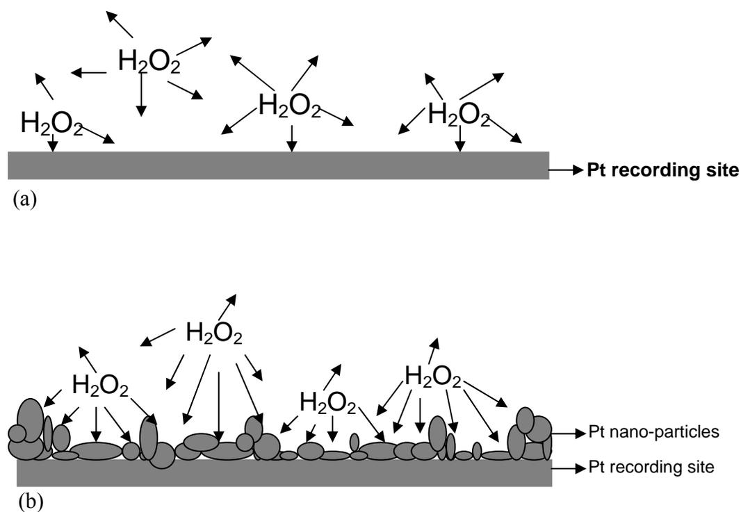
**Figure 1.3: Schematic of  $H_2O_2$  sensing process on (a) bare Pt electrode (b) high surface area electrode (Pt-black nanostructures deposited in the Pt surface). The addition of a high surface area coating increases the number of active sites for  $H_2O_2$  oxidation.**
