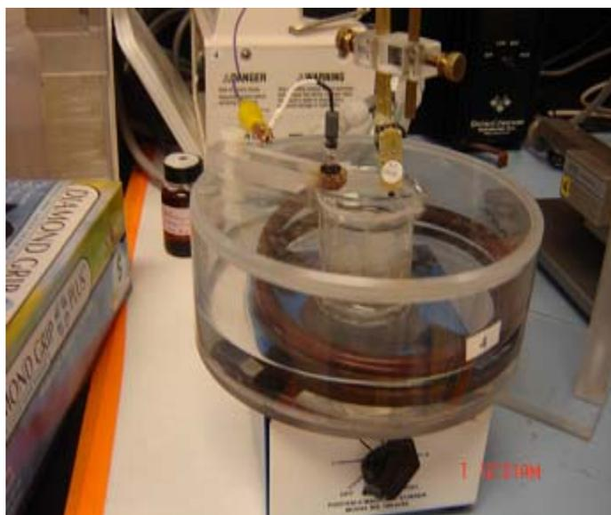
**Figure 3.3: Photograph of microelectrode immersed in calibration chamber. The calibration solution is maintained at 37°C for Glutamate calibration.**
