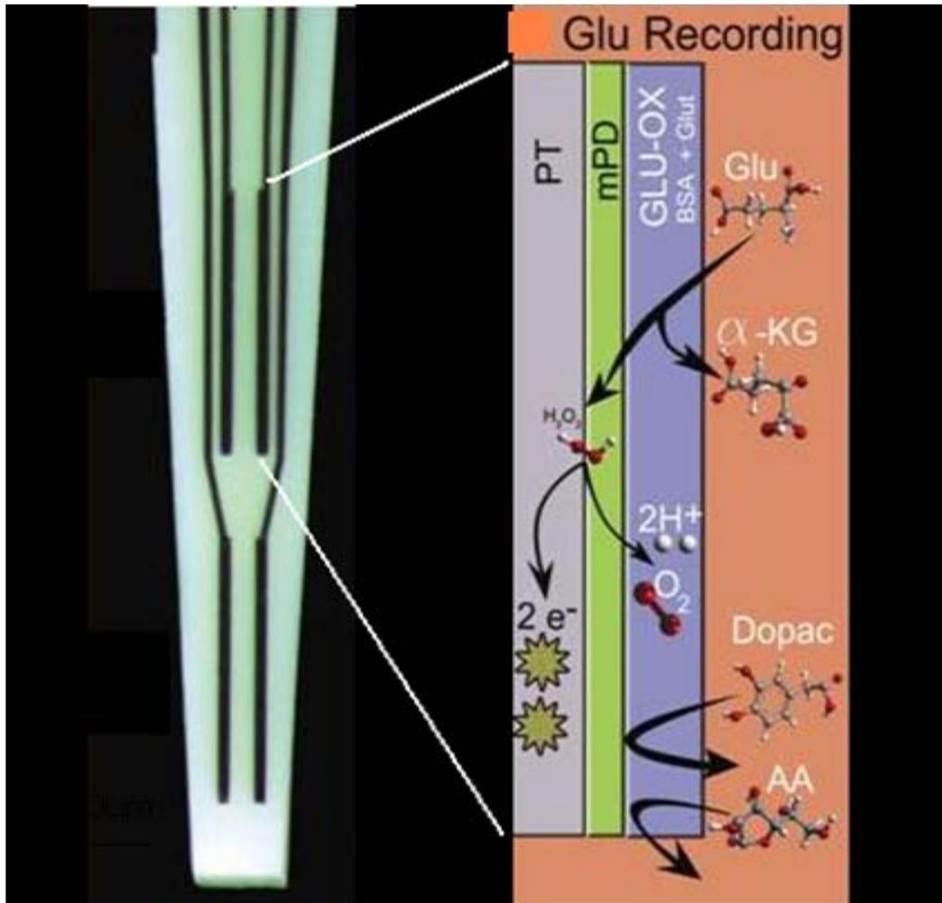
**Figure 1.2: Schematic of the different layers present on the Pt recording site in order to measure glutamate.**
