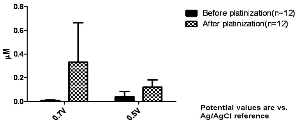
Figure 4.11: Comparative graphs depicting lower electrode potential improves the detection limit of the electrode.
