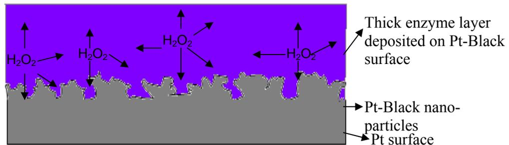
**Figure 4.16(a): Schematic diagram depicting thick enzyme layer over Pt-Black surface. All the peroxide produced is not completely captured by the rough electrode surface**
