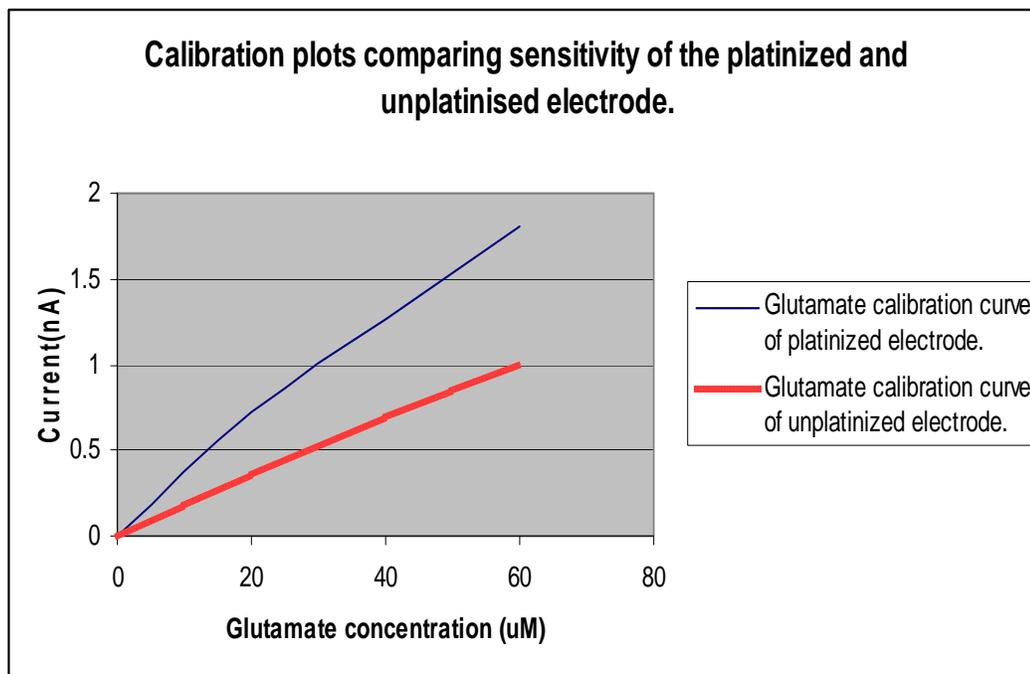
**Figure 4.18: Calibration curves for bare platinum electrode and Pt-Black deposited electrode.**
