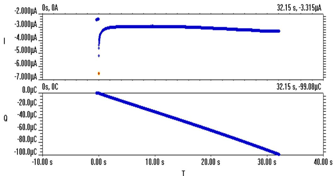
**Figure 4.3: Plots of current and cumulative charge vs. time during electrodeposition.**
