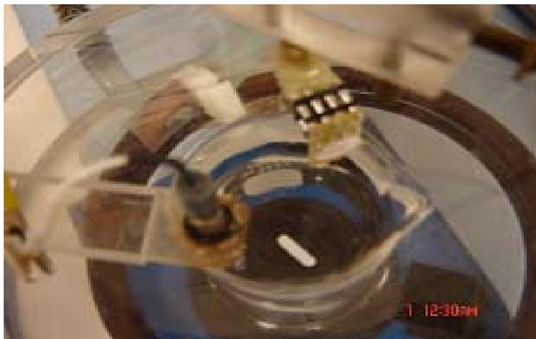
**Figure 3.1: Photograph of microelectrode immersed in calibration chamber. The solution is maintained at room temperature for  $\text{H}_2\text{O}_2$  calibration**
