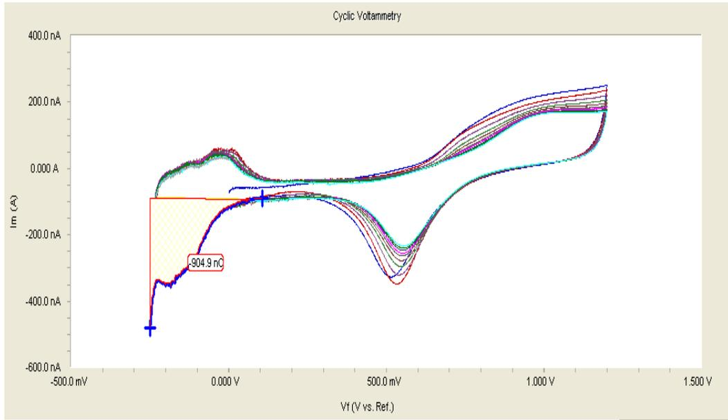
**Figure 4.6: Cyclic voltammogram of platinized recording site. A charge density of  $2\text{Ccm}^{-2}$  was used for Pt-black deposition. The charge in the shaded area depicts adsorption of one hydrogen atom on each Pt atom of the recording surface.**
