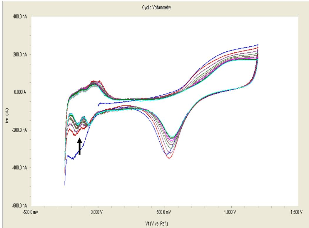
**Figure 4.9: Cyclic voltammetry of platinized recording site. The charge density of  $2 \text{ Ccm}^{-2}$  was used for deposition. The calculated roughness factor of the recording site with nano-particle deposition was  $\sim 86$ . The voltammogram takes some time to stabilize and produce sharp adsorption peaks as shown by the upward arrow.**
