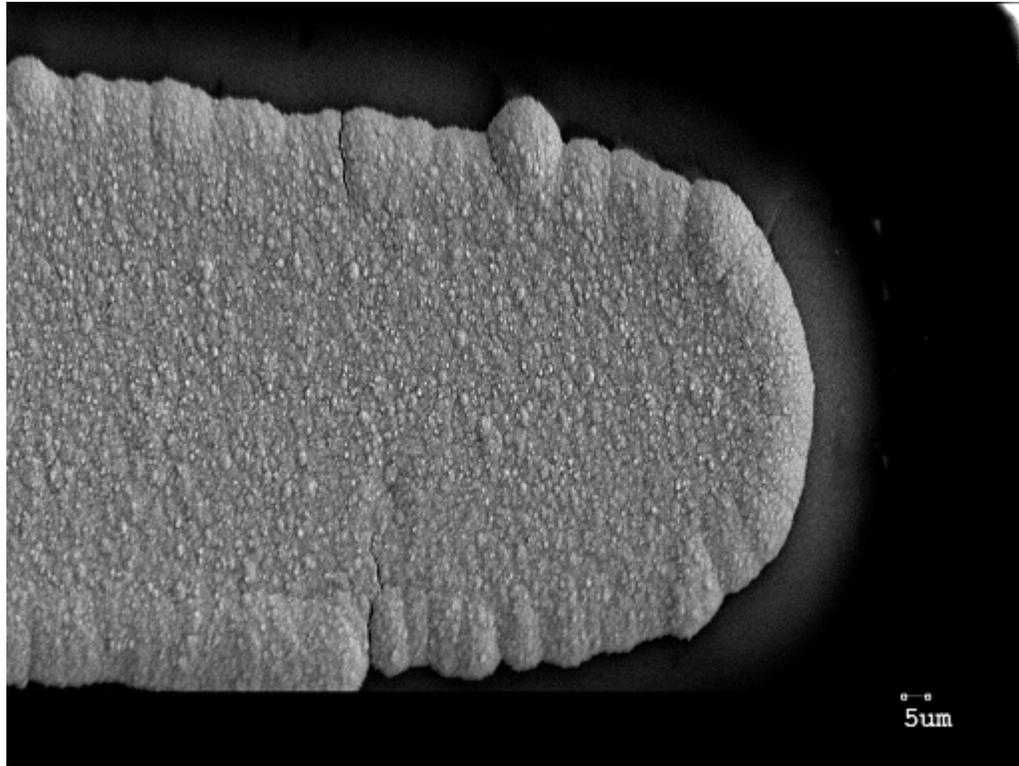
**Figure 4.1: Scanning electron microscope image of platinized recording surface ( $15 \times 333 \mu\text{m}^2$ )**
