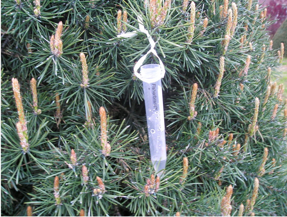
Figure 2.2. A spore trap hung beneath an elongating Scots pine Christmas tree candle in the spring of 2007.
