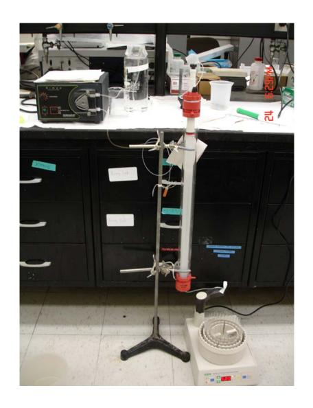
Figure 2.4. A typical gel filtration chromatography system (a pump, a column and a fraction collector)
