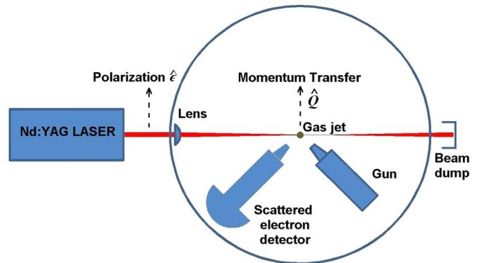
FIG. 1. Schematic of the laser-assisted electron-scattering apparatus.
