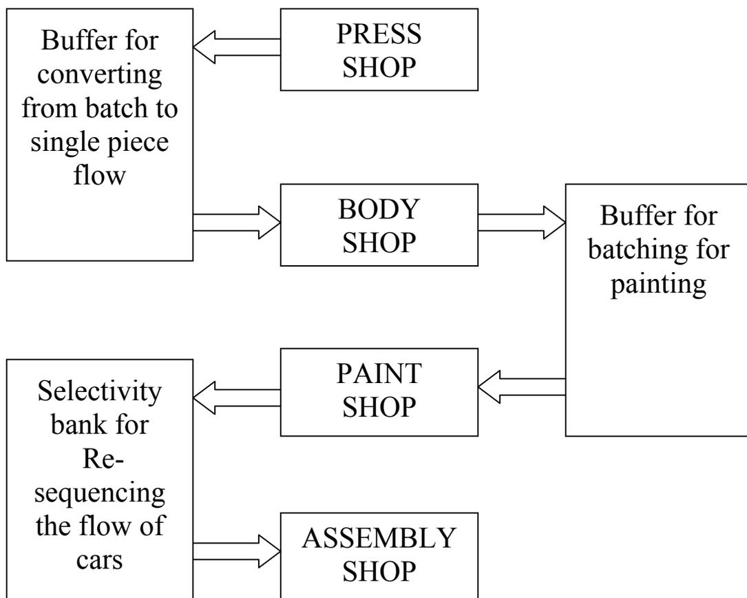
Figure 1.1: General Production Flow in an Automotive Plant
