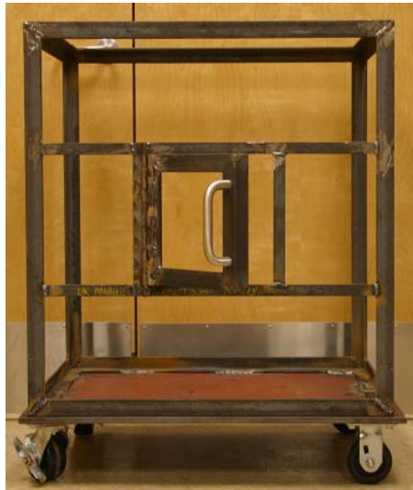
Figure 5.3 Scale Model Furnace Frame
