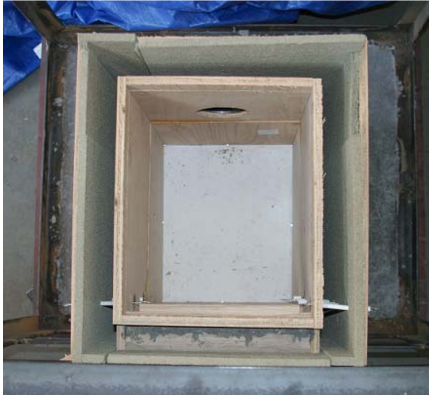
Figure 5.6 Furnace Molds- Top View with Insulation Blocks Inside
