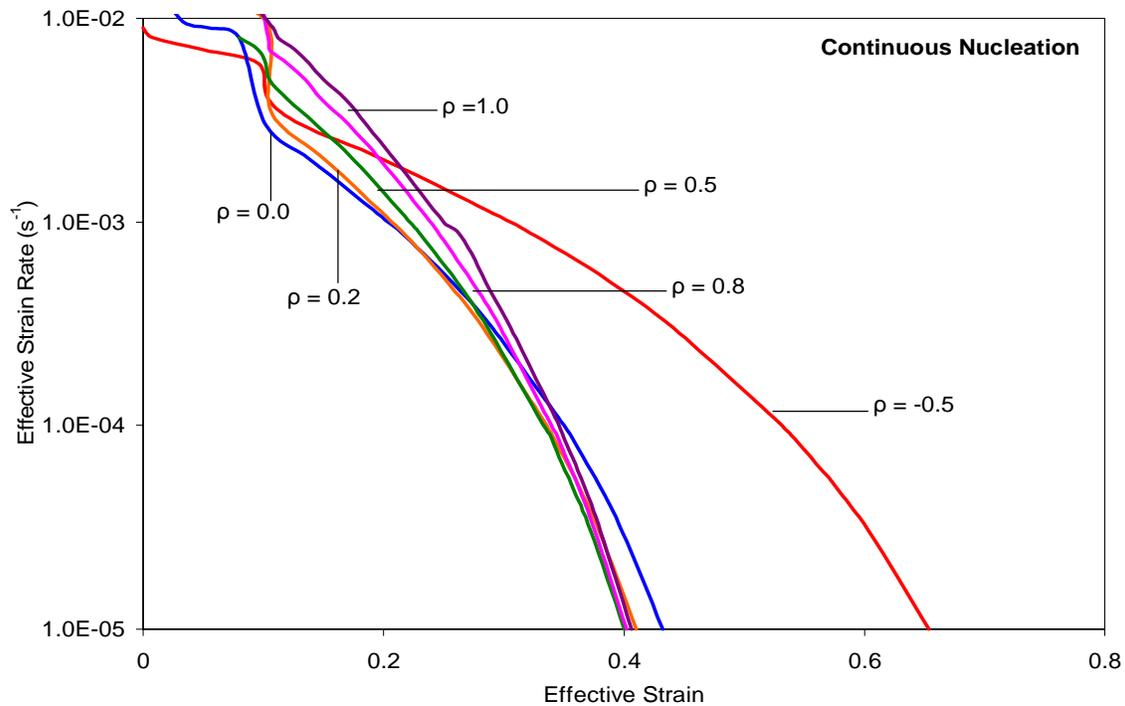
Figure 4-17 Effect of biaxiality ratio ( $\rho$ ) on the optimum forming paths for SP CDA 638 alloy @  $d_0 = 1.3$  microns,  $m = 0.45$ ,  $p=2.4$ ,  $f_{ao}^P = 0.03$  and  $\epsilon_n = 0.1$ ,  $f_{ao}^N = 0.05$  (continuous nucleation)
