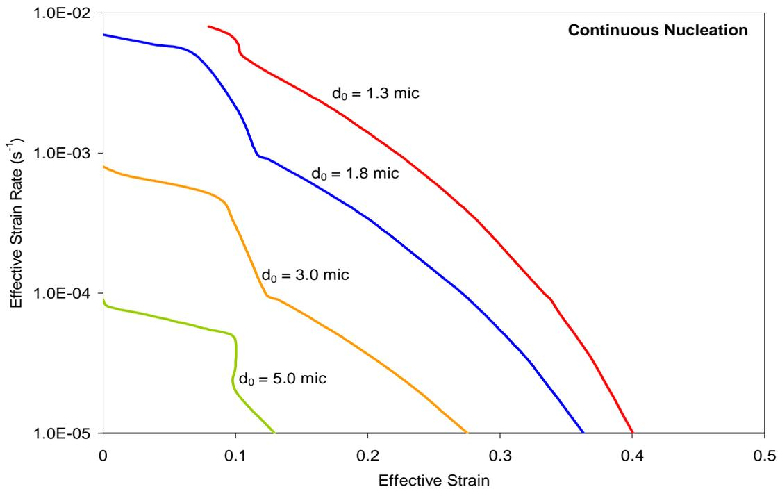
Figure 4-3 Effect of initial grain size on the Optimum forming paths of SP CDA 638 @  $m=0.45$ ,  $p=2.4$ ,  $\epsilon_n=0.1$ ,  $f_{ao}^P = 0.03$ , (continuous nucleation)  $f_{ao}^N = 0.05$  and  $\rho = 0.5$
