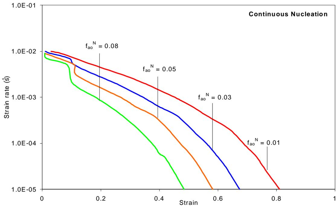
Figure 3-23 Effect of Pre-existing + varying Nucleating (continuous) cavities on the Optimum Forming paths of SP CDA 638 @  $d_o=1.3$ microns,  $\epsilon_n=0.1$ ,  $p=2.4$ ,  $f_{ao}^P=0.05$ ,  $m=0.45$
