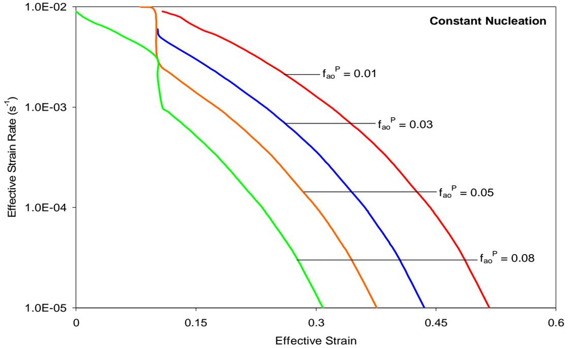
Figure 4-8 Effect of pre-existing cavities on the Optimum Forming paths of SP CDA 638
