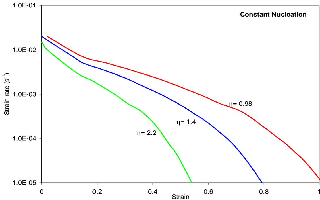
Figure 3-28 Effect of void growth parameter on the optimum forming path of CDA 638 @  $d_o = 1.3\mu$ ,  $m = 0.45$ ,  $p = 2.4$ ,  $\epsilon_n = 0.1$ ,  $f_{ao}^P = 0.03$  and  $f_{ao}^N = 0.05$  (constant nucleation case)
