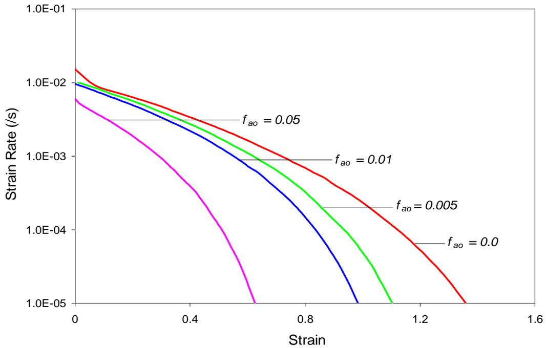
Figure 3-13 Effect of Pre-existing cavities on the Optimum Forming paths of SP CDA 638 @  $d_o=1.3$ microns,  $p=2.4$  and  $m=0.45$
