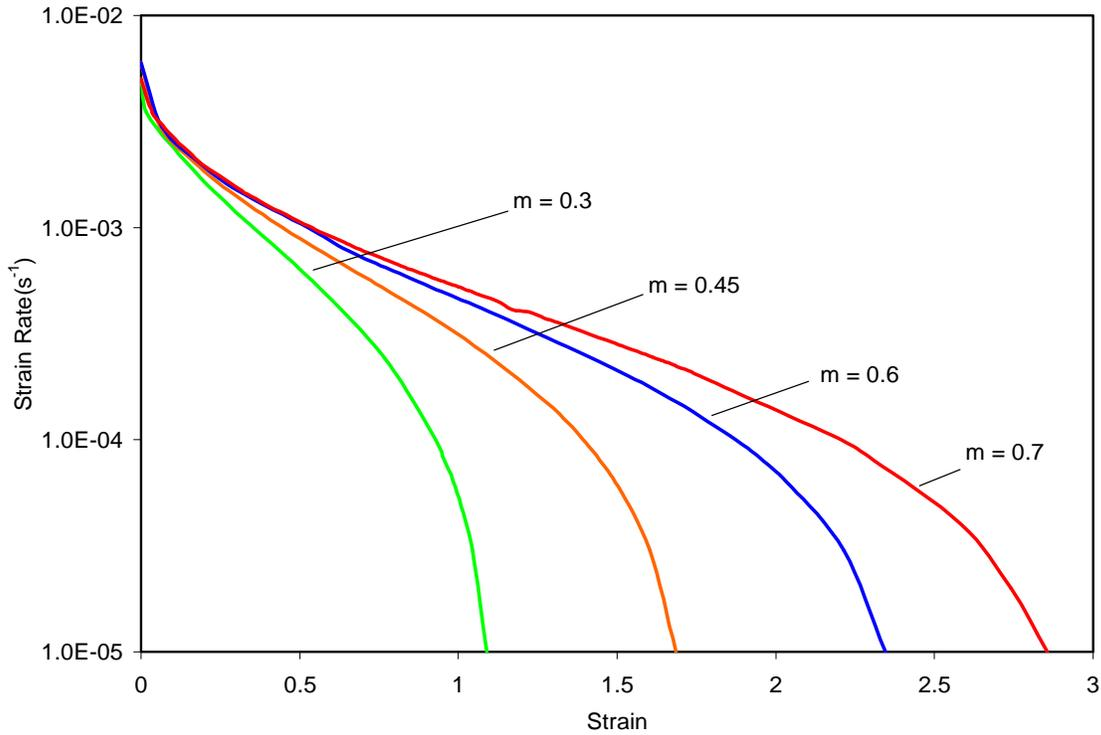
Figure 3-14 Effect of ‘m’ on the Optimum Forming paths of SP Ti6Al4V @  $d_o=4\mu$ ,  $f_{a0}^P=0.05$
