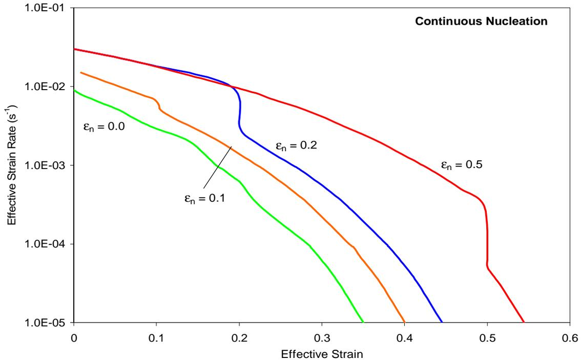
Figure 4-19 Effect of nucleation strain ( $\epsilon_n$ ) on the optimum forming paths for SP CDA 638 alloy @  $d_o = 1.3$  mic,  $\rho=0.5$ ,  $m = 0.45$ ,  $p=2.4$ ,  $f_{ao}^P = 0.03$ ,  $f_{ao}^N = 0.05$  (continuous nucleation)
