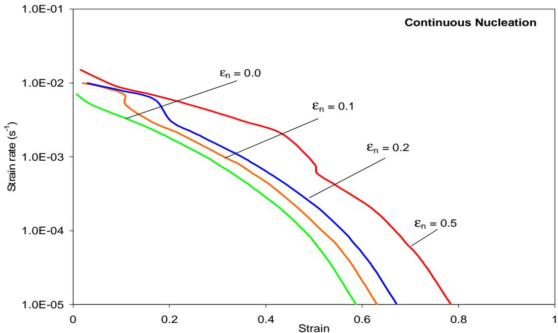
Figure 3-25 Effect of Nucleation strain ( $\epsilon_n$ ) on the Optimum Forming paths of CDA 638 @  $d_0=1.3\mu$ ,  $m=0.45$ ,  $p=2.4$ ,  $f_{a0}^P=0.03$  and  $f_{a0}^N=0.05$  (continuous nucleation case)
