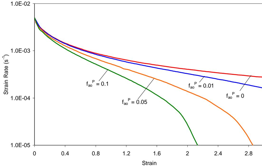
Figure 3-11 Effect of Pre-existing cavities on the Optimum Forming paths of SP Ti6Al4V @  $d_o=4\text{microns}$ ,  $m=0.7$ ,  $p=3.0$
