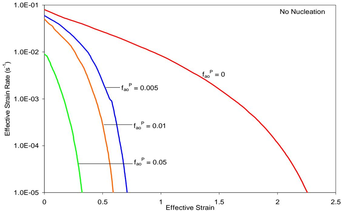
Figure 4-7 Effect of pre-existing cavities on the Optimum Forming paths of SP CDA 638 @  $d_0 = 1.3 \mu\text{m}$ ,  $p = 2.4$ ,  $m = 0.45$
