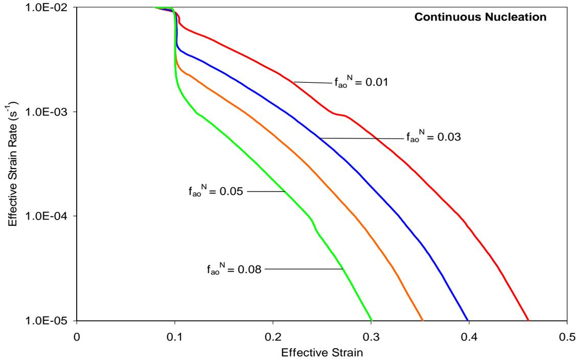
Figure 4-13 Effect of nucleating (continuous) and pre-existing cavities on the Optimum Forming paths of SP CDA 638 @  $d_o=1.3$  microns,  $p=2.4$ ,  $\epsilon_n=0.1$ ,  $f_{ao}^P=0.05$  and  $\rho=0.5$
