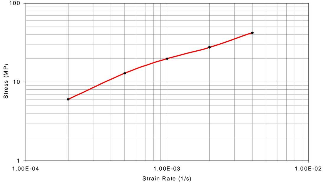
Figure 3-1 Stress vs.- Strain rate curves for SP Ti-6Al-4V @ 900°C in region II
