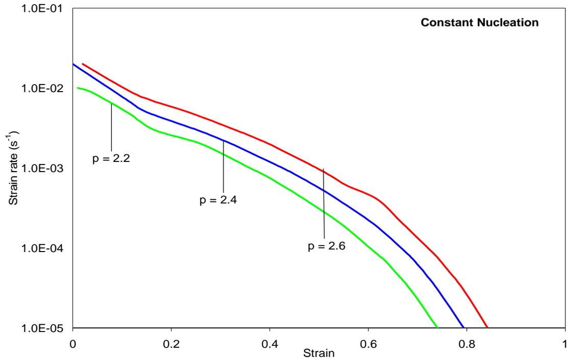
Figure 3-26 Effect of 'p' on the Optimum forming paths of SP CDA 638 @  $d_o=1.3\mu$ ,  $m=0.45$ ,  $\epsilon_n=0.1$ ,  $f_{ao}^P=0.03$  and  $f_{ao}^N=0.05$  (constant nucleation case)
