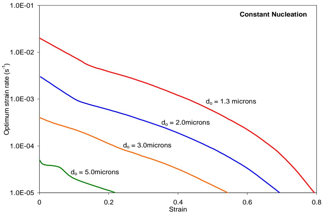
Figure 3-9 Effect of initial grain size on the Optimum forming paths of SP CDA 638 @  $p=2.4$ ,  $m=0.45$ ,  $f_{ao}^P=0.03$ ,  $\epsilon_n=0.1$  and  $f_{ao}^N=0.05$
