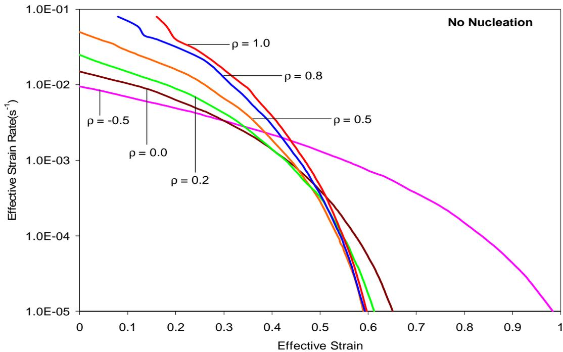
Figure 4-15 Effect of biaxiality ratio ( $\rho$ ) on the optimum forming paths for SP CDA 638 alloy @  $d_0 = 1.3$  microns,  $m = 0.45$ ,  $p=2.4$ ,  $f_{a0}^P = 0.01$  and no nucleation
