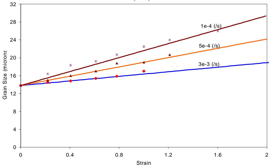
Figure 3-4 Fitting grain growth model to experimental data [41] for AA 5083
