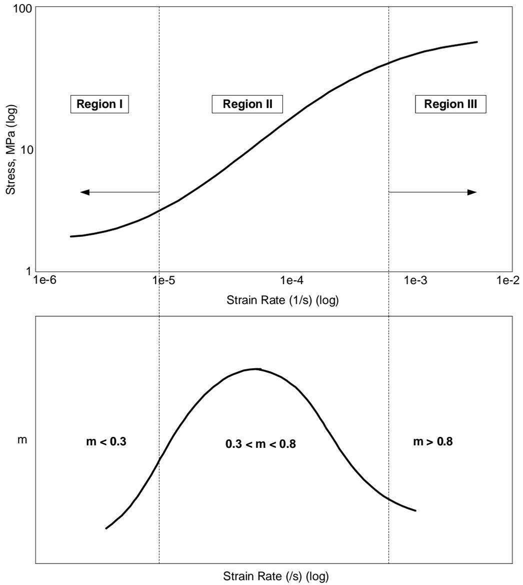
Figure 2-1 Typical Stress Strain rate relation for SP materials. Dependence of (a) flow stress, and (b) strain rate sensitivity index on strain rate
