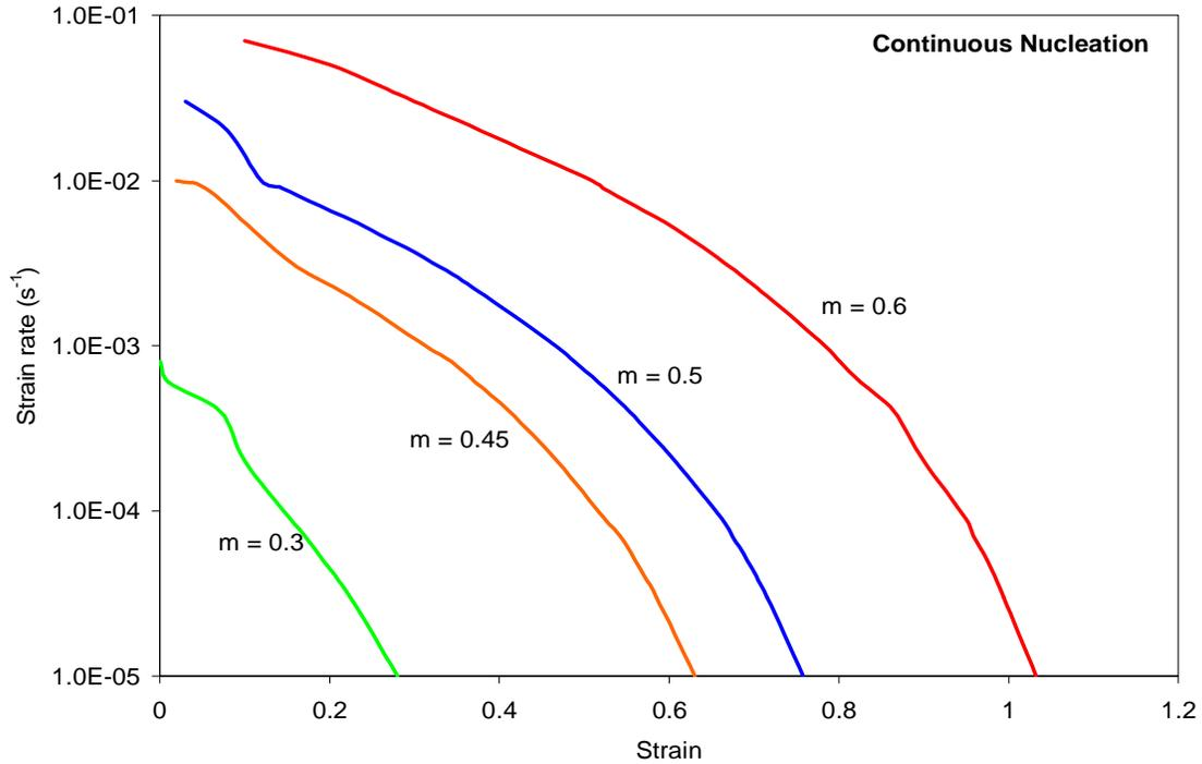
Figure 3-16 Effect of ‘m’ on Optimum Forming paths of CDA 638 @  $d_o=1.3\mu$ ,  $p=2.4$ ,  $\epsilon_n = 0.1$ ,  $f_{ao}^P=0.05$  and (continuous nucleation)  $f_{ao}^N=0.03$
