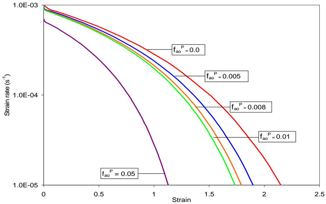
Figure 3-12 Effect of Pre-existing cavities on the Optimum Forming paths of SP AA 5083 @  $d_o=13$  microns and  $m=0.6$
