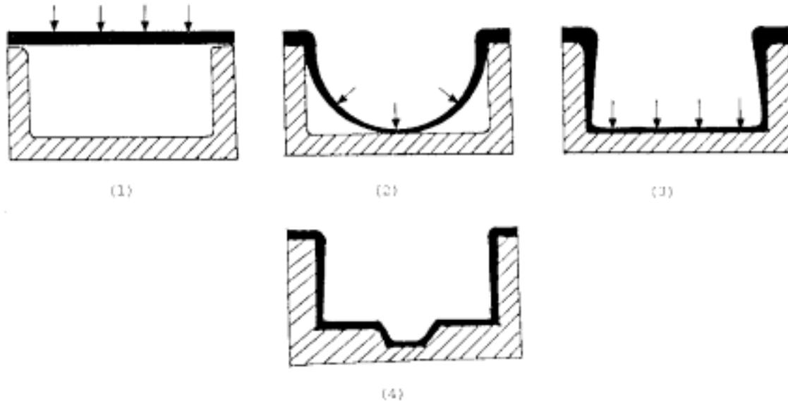
Figure 1-1 Schematic of Simple Female Forming [1]
