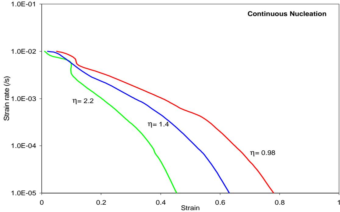
Figure 3-29 Effect of void growth parameter on the optimum forming path of CDA 638 @  $d_0=1.3\mu$ ,  $m=0.45$ ,  $p=2.4$ ,  $\epsilon_n=0.1$ ,  $f_{ao}^P=0.03$  and  $f_{ao}^N=0.05$  (continuous nucleation case)
