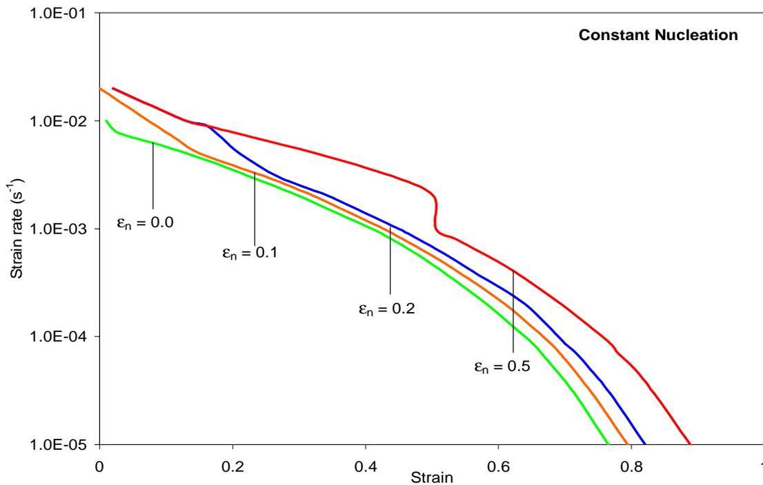
Figure 3-24 Effect of Nucleation strain ( $\epsilon_n$ ) on the Optimum Forming paths of CDA 638 @  $d_o=1.3\mu$ ,  $m=0.45$ ,  $p=2.4$ ,  $f_{ao}^P=0.03$  and  $f_{ao}^N=0.05$  (constant nucleation case)
