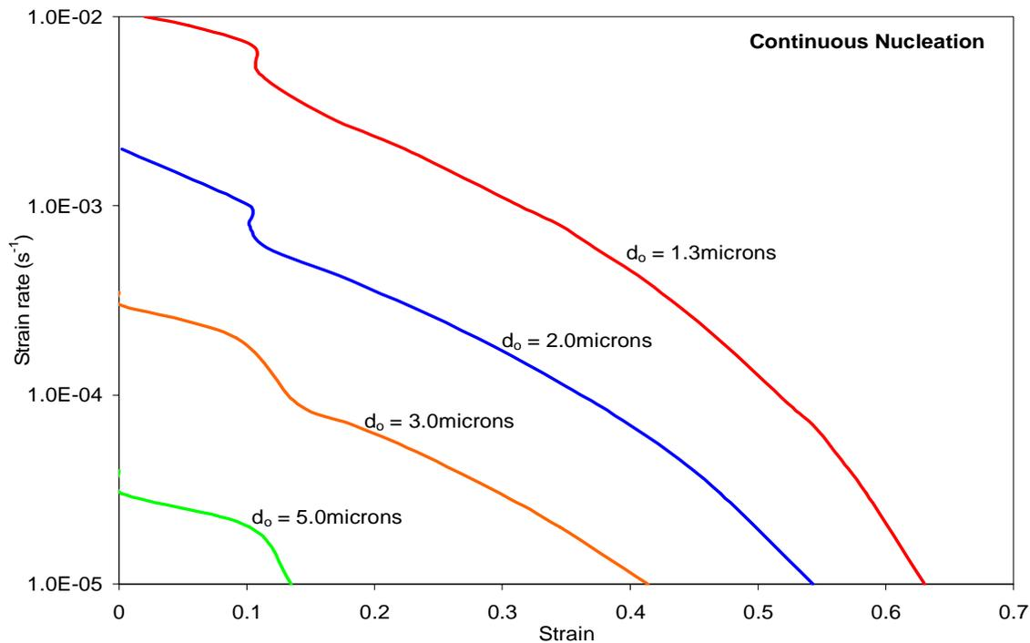
Figure 3-10 Effect of initial grain size on the Optimum forming paths of SP CDA 638 @  $p=2.4, m=0.45, f_{ao}^P=0.03, \epsilon_n=0.1$  and  $f_{ao}^N=0.05$
