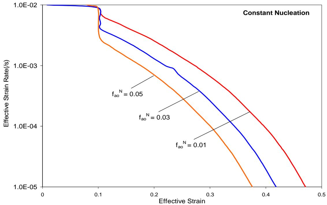
Figure 4-12 Effect of nucleating (constant) and pre-existing cavities on the Optimum Forming paths of SP CDA 638 @  $d_o=1.3$  microns,  $p=2.4$ ,  $\epsilon_n=0.1$ ,  $f_{ao}^P=0.05$  and  $\rho=0.5$
