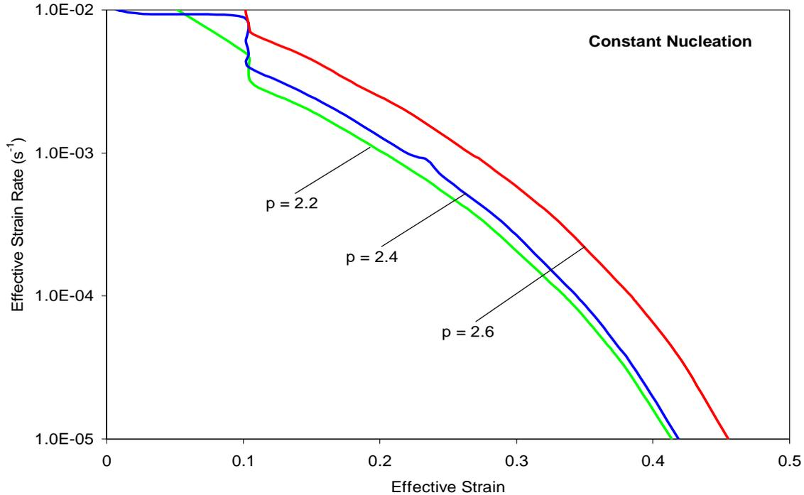
Figure 4-20 Effect of ‘p’ on the optimum forming paths for SP CDA 638 alloy @  $d_0 = 1.3$  microns,  $\rho=0.5$ ,  $m = 0.45$ ,  $f_{a0}^P = 0.03$ ,  $f_{a0}^N = 0.05$  (constant nucleation)
