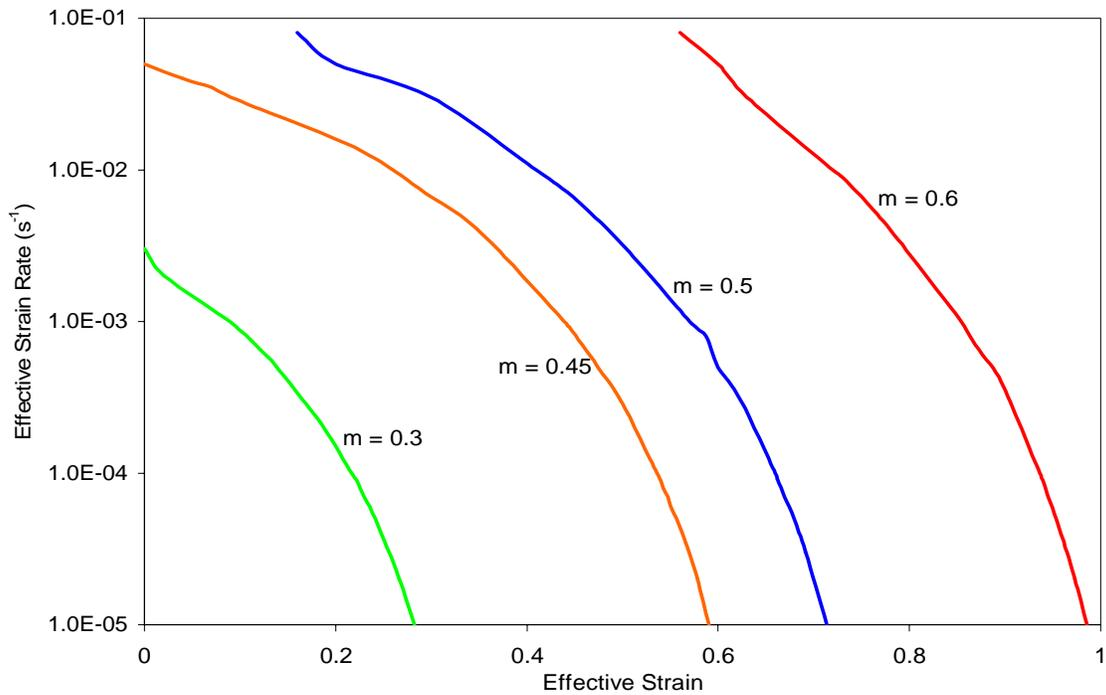
Figure 4-4 Effect of ‘m’ on the Optimum Forming paths of SP CDA 638 @
