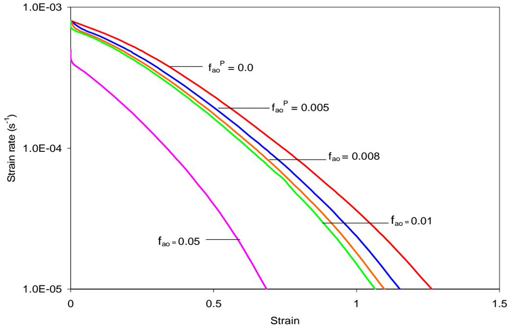
Figure 3-17 Effect of varying  $f_{ao}^P$  on Optimum Forming paths with ‘m’ varying during deformation as a function of  $\dot{\epsilon}$
