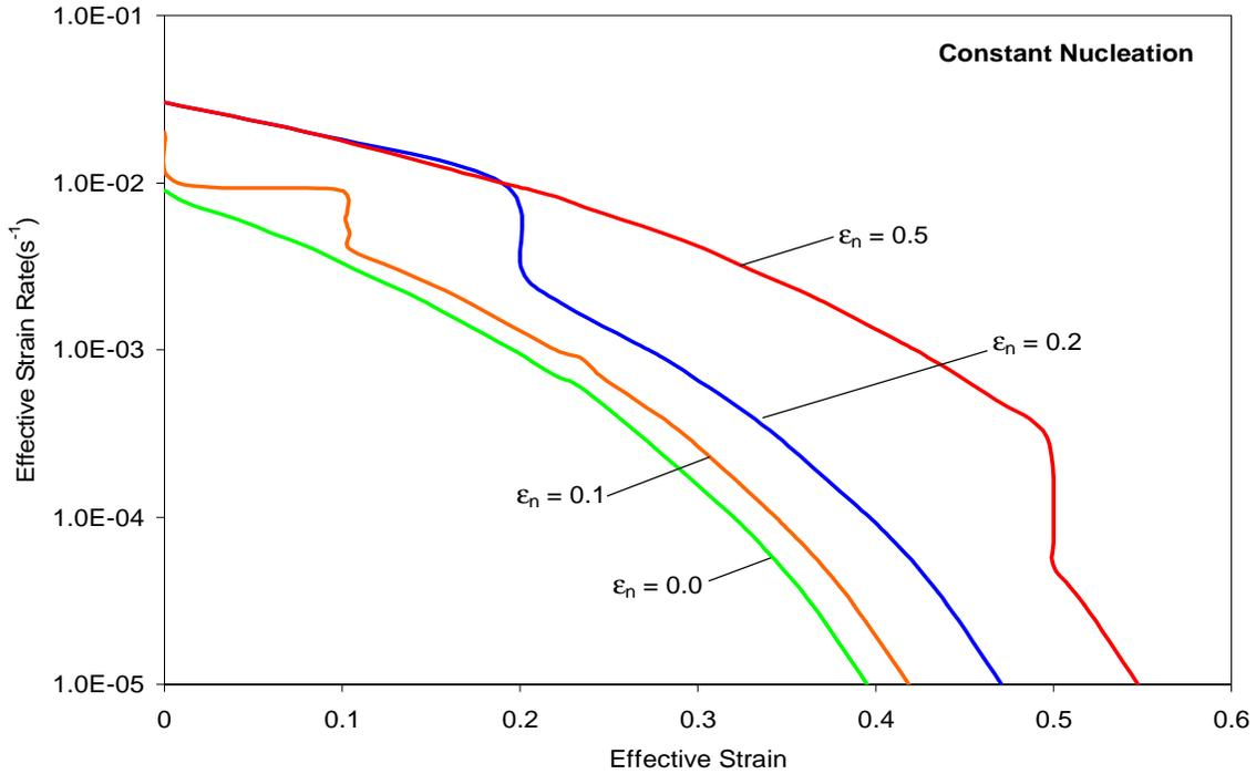
Figure 4-18 Effect of nucleation strain ( $\epsilon_n$ ) on the optimum forming paths for SP CDA 638 alloy @  $d_o = 1.3$  mic,  $\rho=0.5$ ,  $m = 0.45$ ,  $p=2.4$ ,  $f_{ao}^P = 0.03$ ,  $f_{ao}^N = 0.05$  (constant nucleation)
