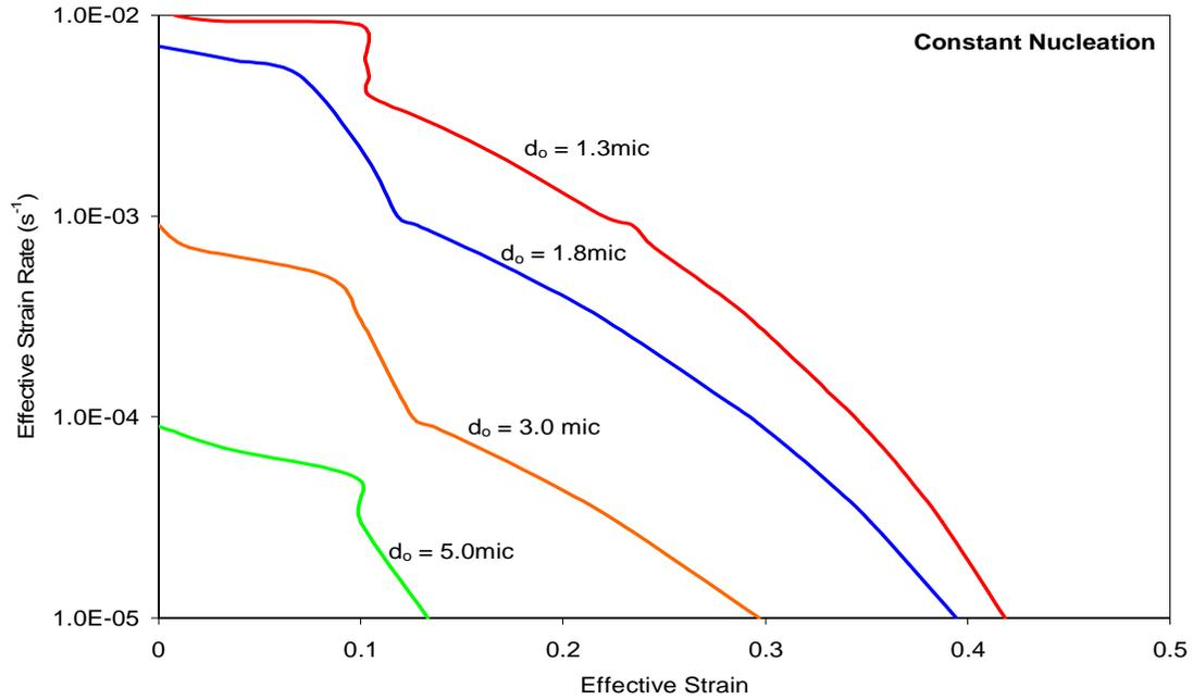
Figure 4-2 Effect of initial grain size on the Optimum forming paths of SP CDA 638 @  $m=0.45$ ,  $p=2.4$ ,  $\epsilon_n=0.1$ ,  $f_{ao}^P = 0.03$ , (constant nucleation)  $f_{ao}^N = 0.05$  and  $\rho = 0.5$
