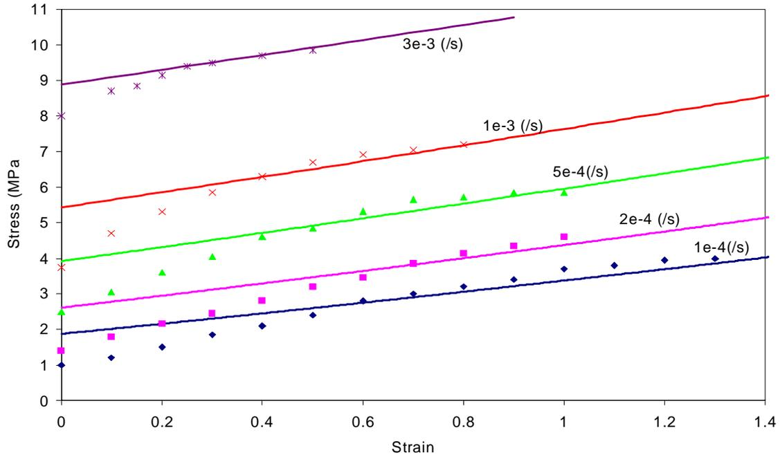
Figure 3-3 Stress vs.-Strain curves for AA 5083 [Fitting the model (line) to experimental values (dots)]
