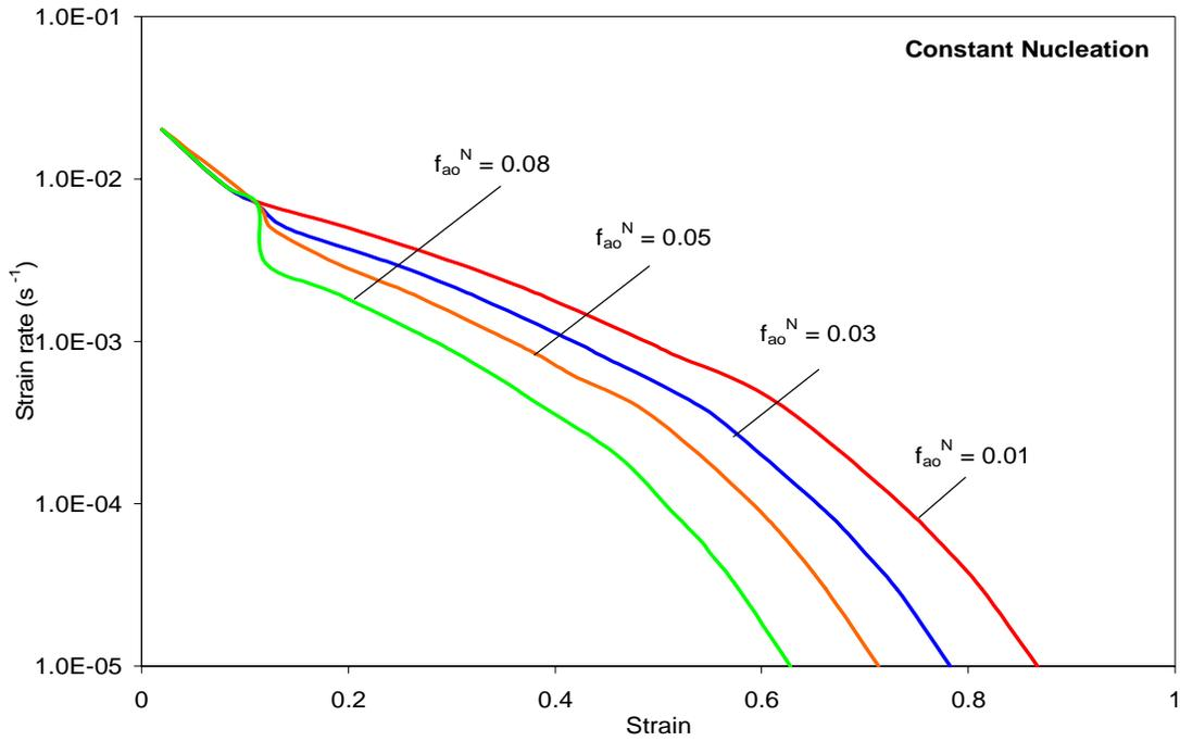
Figure 3-22 Effect of Pre-existing + varying Nucleating (constant) cavities on the Optimum Forming paths of SP CDA 638 @  $d_o=1.3$ microns,  $\epsilon_n=0.1$ ,  $p=2.4$ ,  $f_{ao}^P=0.05$  &  $m=0.45$
