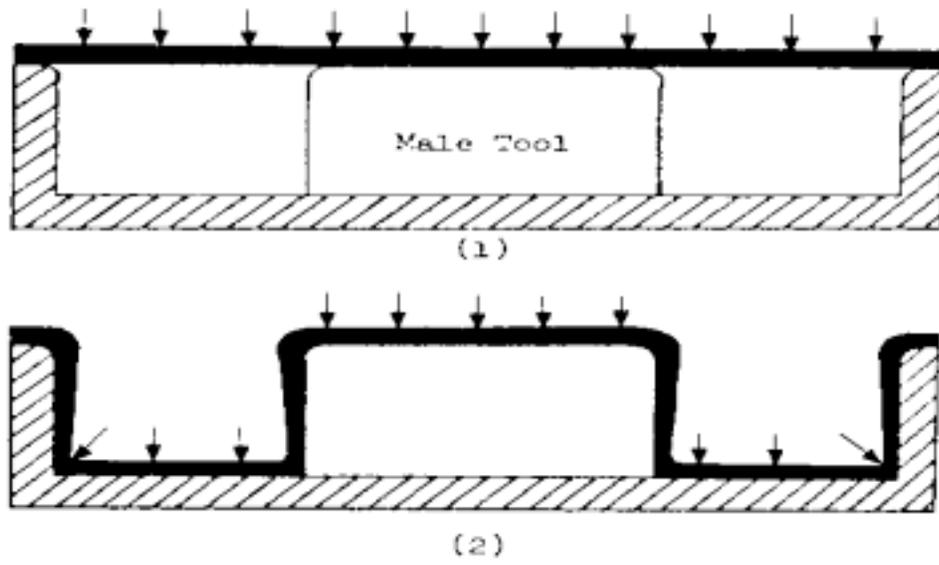
Figure 1-2 Schematic of Female Drape Forming [1]
