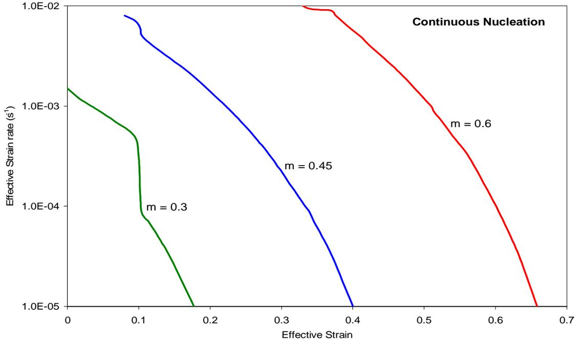
Figure 4-6 Effect of 'm' on the Optimum Forming paths of SP CDA 638 @  $d_o = 1.3$  microns,  $p=2.4$ ,  $\epsilon_n=0.1$ ,  $f_{ao}^P = 0.03$ , (continuous nucleation)  $f_{ao}^N = 0.05$  and  $\rho = 0.5$
