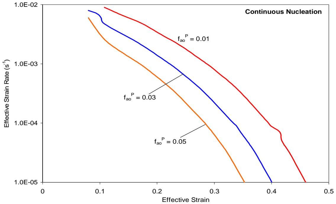
Figure 4-9 Effect of pre-existing cavities on the Optimum Forming paths of SP CDA 638
