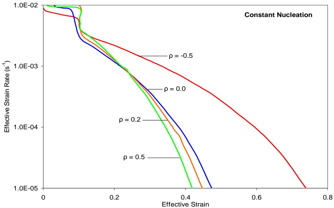
Figure 4-16 Effect of biaxiality ratio ( $\rho$ ) on the optimum forming paths for SP CDA 638 alloy @  $d_0 = 1.3$  microns,  $m = 0.45$ ,  $p = 2.4$ ,  $f_{ao}^P = 0.03$  and  $\epsilon_n = 0.1$ ,  $f_{ao}^N = 0.05$  (constant nucleation)
