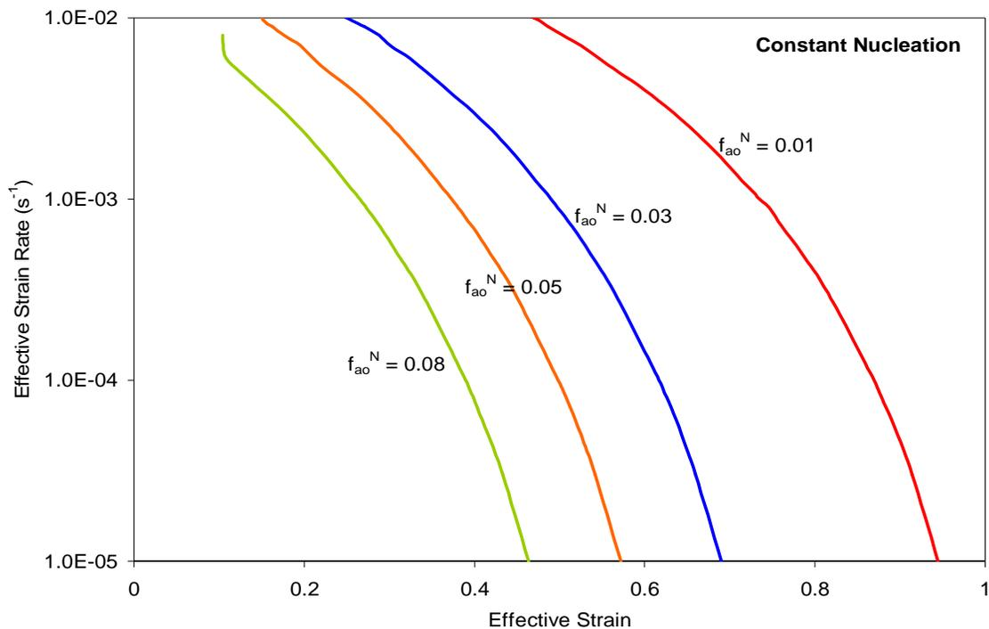
Figure 4-10 Effect of nucleating (constant) cavities on the Optimum Forming paths of
