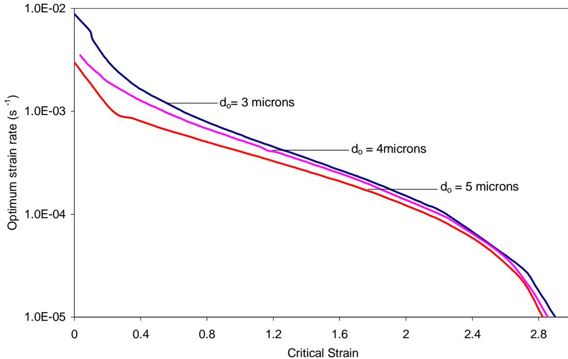
Figure 3-7 Effect of initial grain size on the Optimum forming paths of SP Ti6Al4V @  $m=0.6-0.7$ ,  $f_{ao}^P=0.05$ ,  $p=3.0$
