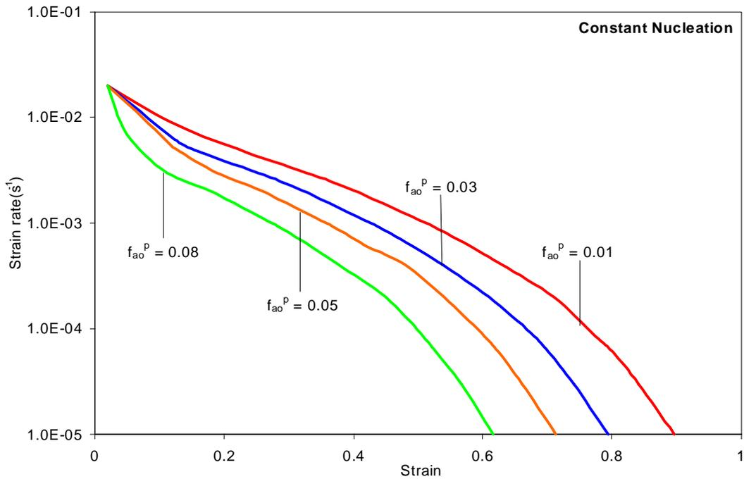
Figure 3-20 Effect of varying Pre-existing + Nucleating (constant) cavities on the Optimum Forming paths of SP CDA 638 @  $d_o=1.3\text{mic}$ ,  $\epsilon_n=0.1$ ,  $p=2.4$ ,  $f_{ao}^N=0.05$  &  $m=0.45$
