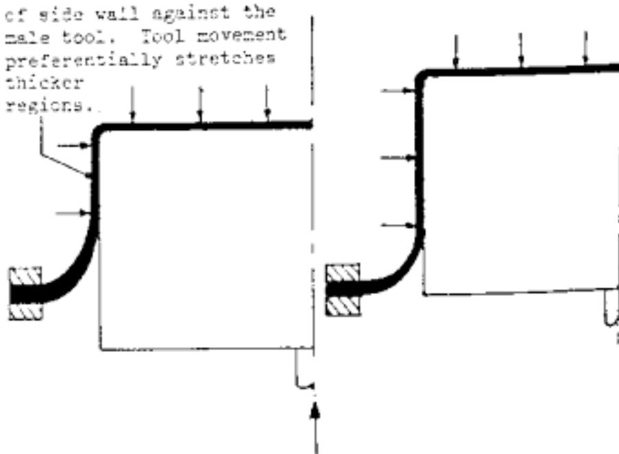
Figure 1-5 Schematic of Snap-Back Forming [1]
