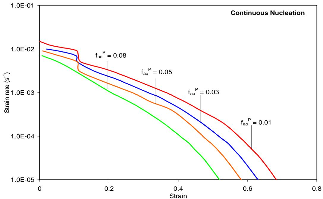
Figure 3-21 Effect of varying Pre-existing + Nucleating (continuous) cavities on the Optimum Forming paths of SP CDA 638 @  $d_0=1.3\text{microns}$ ,  $\epsilon_n=0.1$ ,  $p=2.4$ ,  $f_{ao}^N=0.05$  &  $m=0.45$
