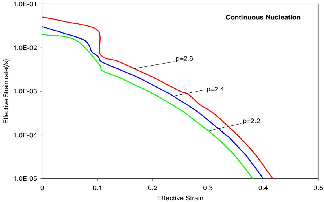
Figure 4-21 Effect of ‘p’ on the optimum forming paths for SP CDA 638 alloy @  $d_o = 1.3$  microns,  $\rho=0.5$ ,  $m = 0.45$ ,  $f_{ao}^P = 0.03$ ,  $f_{ao}^N = 0.05$  (continuous nucleation)
