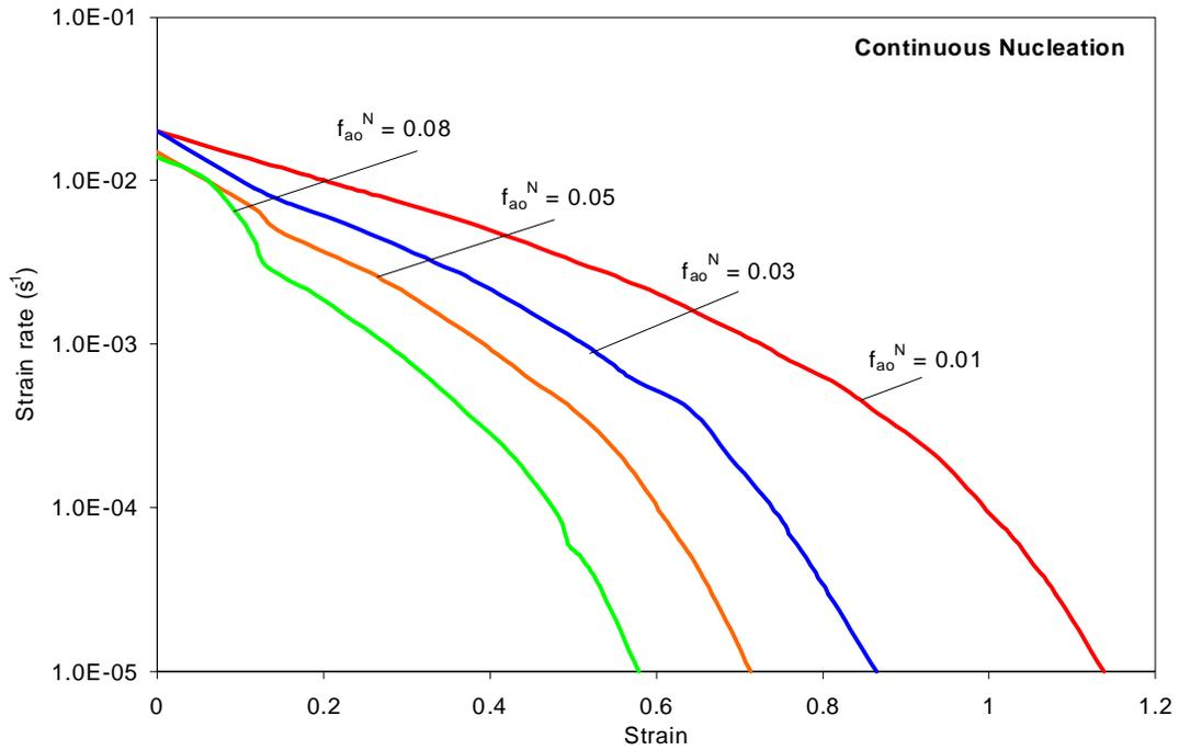
Figure 3-19 Effect of Nucleating (continuous) cavities on the Optimum Forming paths of SP CDA 638 @  $d_o=1.3\text{microns}$ ,  $\epsilon_n=0.1$ ,  $p=2.4$ ,  $f_{ao}^P=0$  and  $m=0.45$
