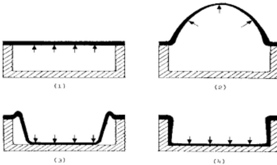
Figure 1-3 Schematic of Reverse Bulging [1]
