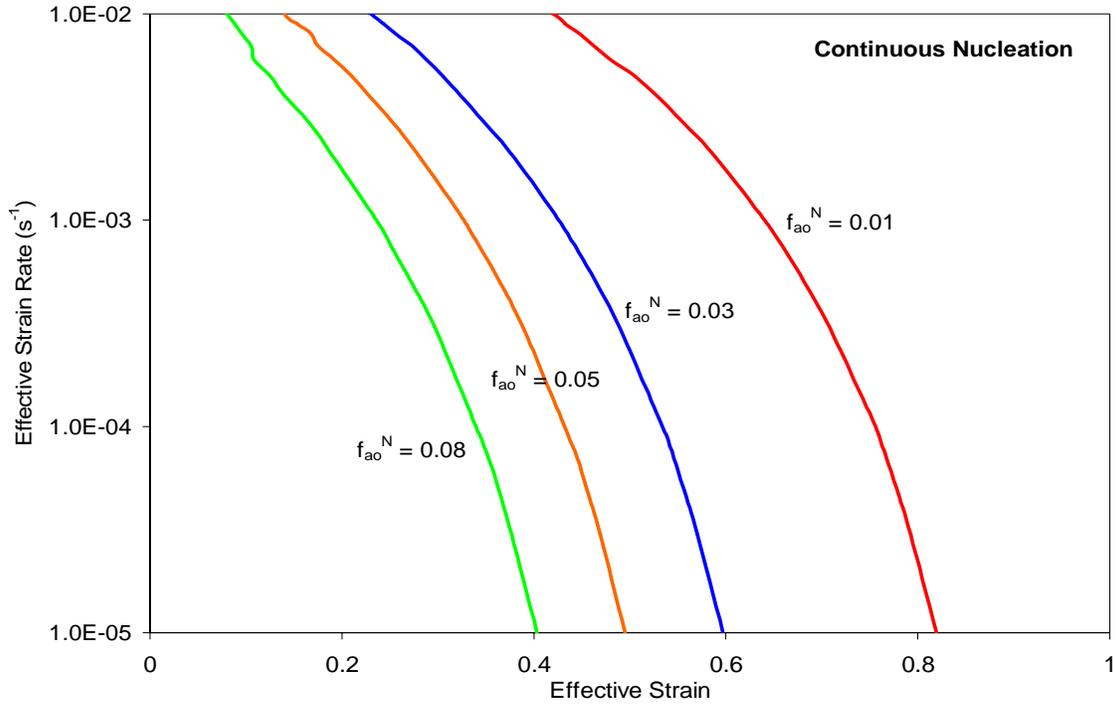
Figure 4-11 Effect of nucleating (continuous) cavities on the Optimum Forming paths of SP CDA 638 @  $d_o=1.3$  microns,  $p=2.4$ ,  $\epsilon_n=0.1$ ,  $f_{ao}^P=0.0$  and  $\rho=0.5$
