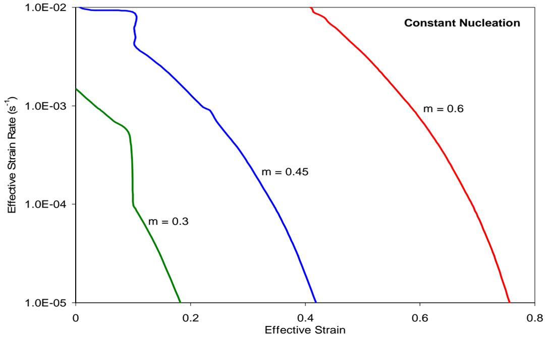
Figure 4-5 Effect of 'm' on the Optimum Forming paths of SP CDA 638 @  $d_o = 1.3$  microns,  $p=2.4$ ,  $\epsilon_n=0.1$ ,  $f_{ao}^P = 0.03$ , (constant nucleation)  $f_{ao}^N = 0.05$  and  $\rho = 0.5$
