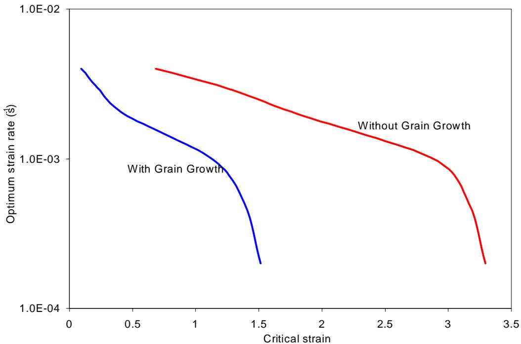
Figure 3-6 Effect of grain growth on the Optimum Forming path of SP Ti6Al4V @  $d_o=4\text{mic}$ ,  $p=3.0$ ,  $f_{ao}^p=0.01$ ,  $m=0.6-0.7$
