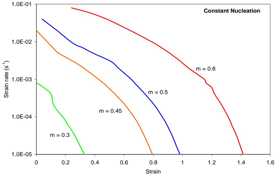
Figure 3-15 Effect of ‘m’ on Optimum Forming paths of CDA 638 @  $d_o=1.3\mu$ ,  $p=2.4$ ,  $\epsilon_n = 0.1$ ,  $f_{ao}^P=0.05$  and (constant nucleation)  $f_{ao}^N=0.03$
