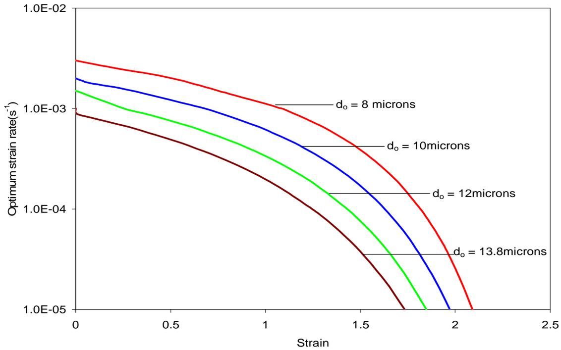
Figure 3-8 Effect of initial grain size on the Optimum forming paths of SP AA 5083 @  $m=0.6$ ,  $f_{ao}^P=0.01$ ,  $p$  and  $c$  are evaluated as function of strain rate
