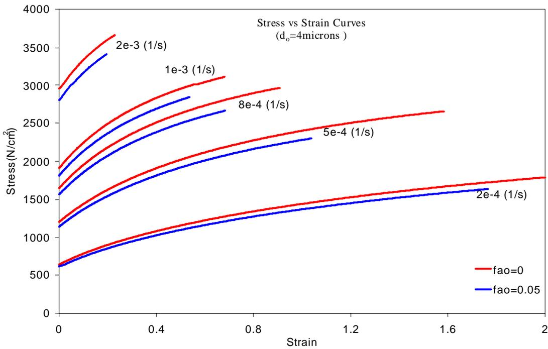
Figure 3-2 Stress vs.- Strain curves for SP Ti-6Al-4V @ 900°C in region II
