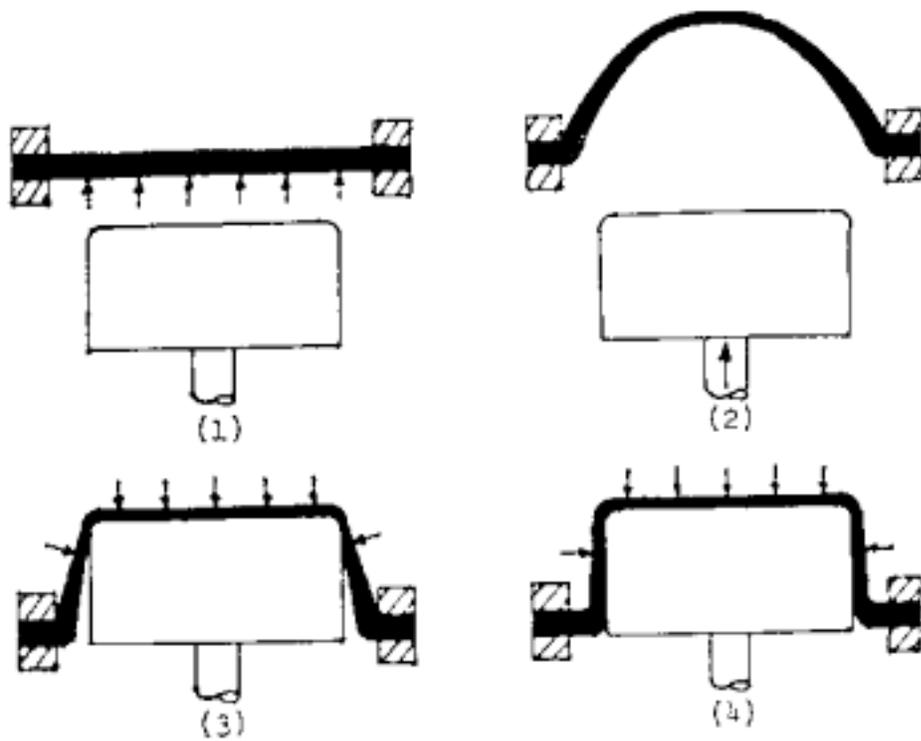
Pressure locks thin regions of side wall against the male tool. Tool movement preferentially stretches thicker regions.
