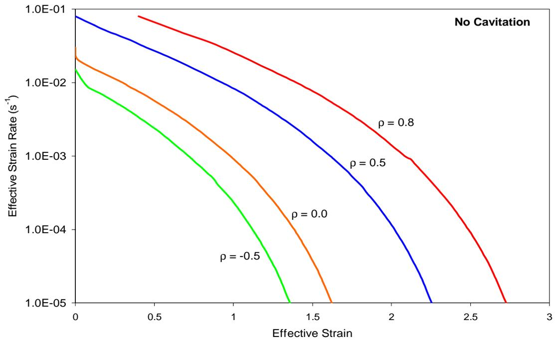
Figure 4-14 Effect of biaxiality ratio ( $\rho$ ) on the optimum forming paths for SP CDA 638 alloy @  $d_0 = 1.3$  microns,  $m = 0.45$ ,  $p=2.4$  and no cavitation
