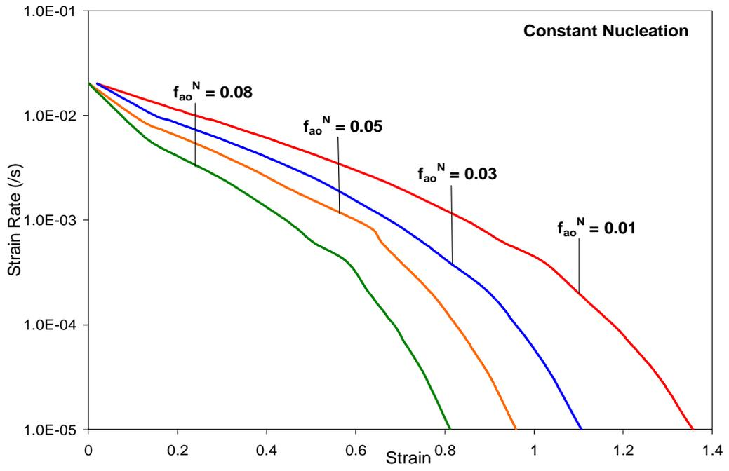
Figure 3-18 Effect of Nucleating (constant) cavities on the Optimum Forming paths of SP CDA
