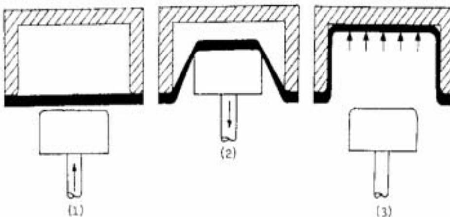
Figure 1-4 Schematic of Plug Assisted Forming [1]
