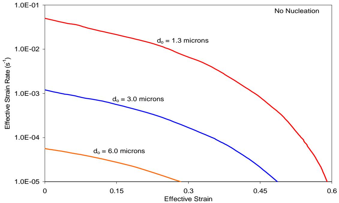
Figure 4-1 Effect of initial grain size on the Optimum forming paths of SP CDA 638 @  $m=0.45$ ,  $p=2.4$ ,  $f_{ao}^P = 0.01$ , and  $\rho = 0.5$
