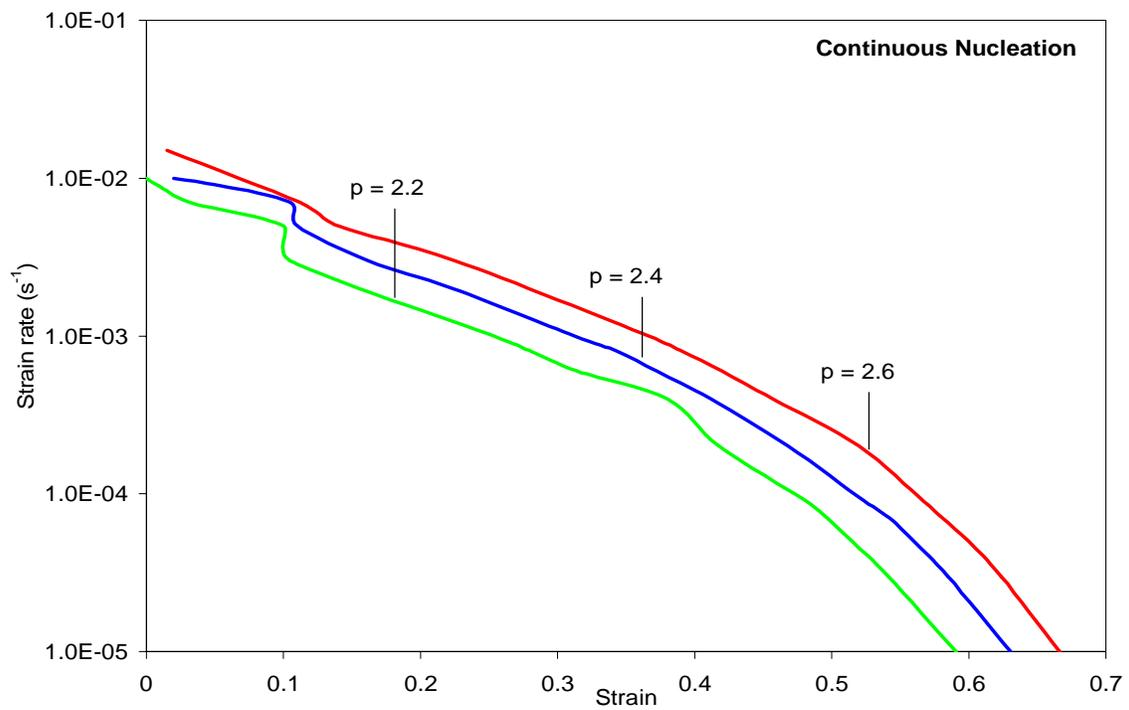
Figure 3-27 Effect of 'p' on the Optimum forming paths of SP CDA 638 @  $d_o=1.3\mu$ ,  $m=0.45$ ,  $\epsilon_n=0.1$ ,  $f_{ao}^P=0.03$  and  $f_{ao}^N=0.05$  (continuous nucleation case)
