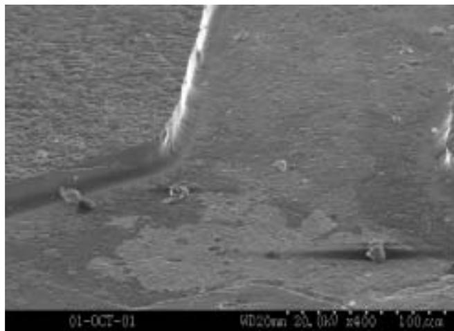
Figure 14: SEM details of an asperity groove [1]
