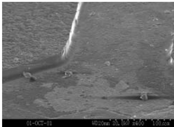
Figure 14: SEM details of an asperity groove [1]
