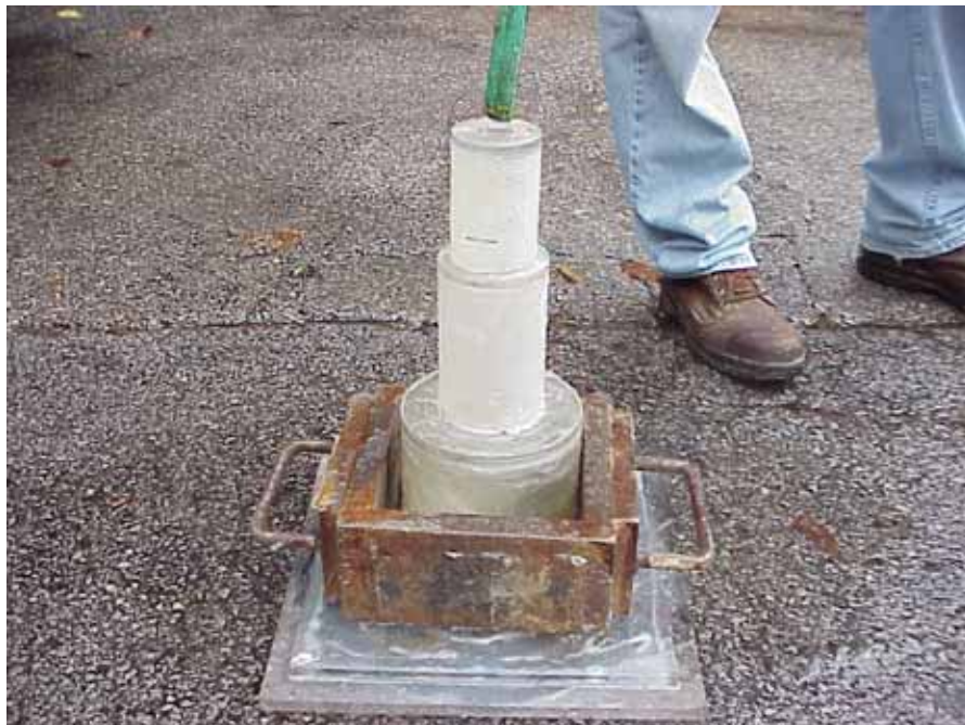
Figure 12. NCAT Permeameter in Place and Being Filled with Water.
