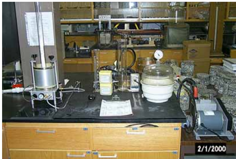
Figure 3. Laboratory Permeability Device.
