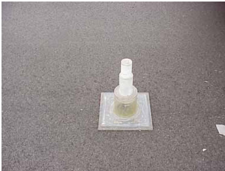
Figure 2. NCAT Field Permeameter.
