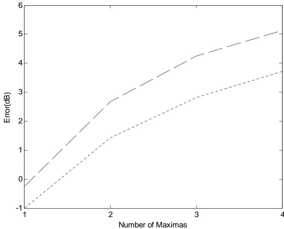
Figure 4.9 Number of maximas vs. Performance Error between Symlets prediction and Subjective results and Gabor prediction and Subjective results for the case of mean. The smallest error occurs at one maximas for Symlet and one for Gabor prediction.
