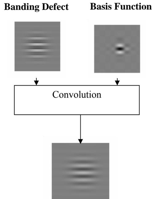
Figure 3.7 Decomposition Process for banding defect patterns
