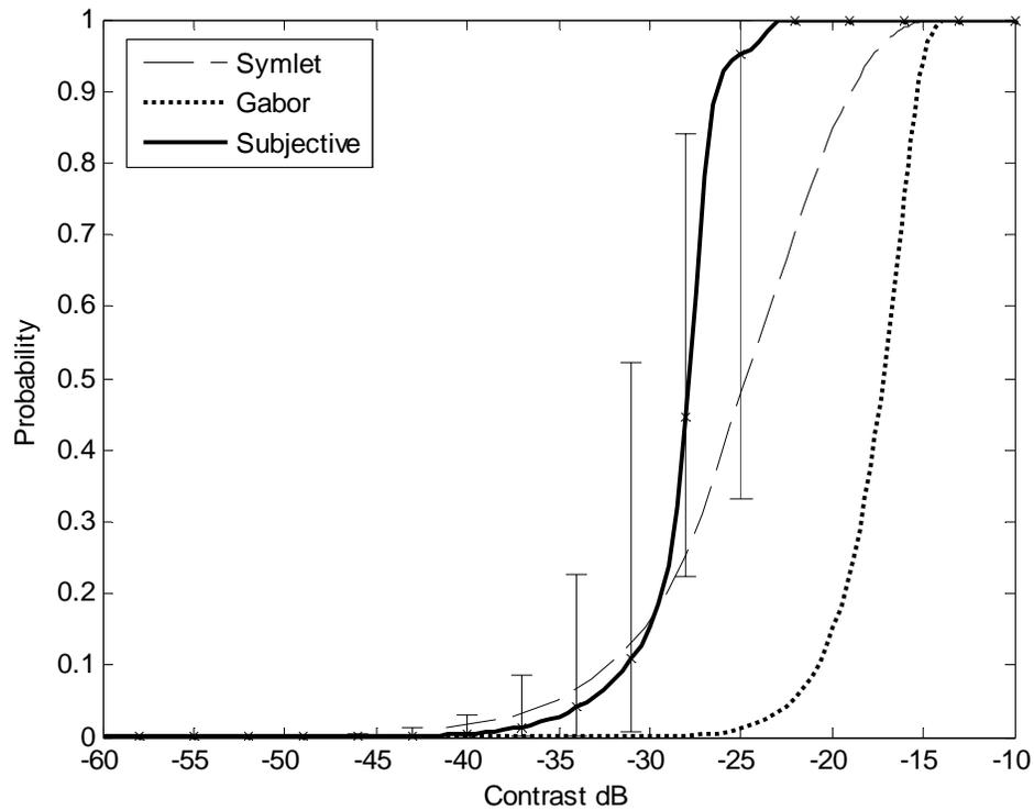
Figure 4. 4 Banding 2-2 using bootstrapping mean, high frequency, large envelope banding pattern. Assumption is made that HVS detects only the absolute maxima when observing a defect pattern
