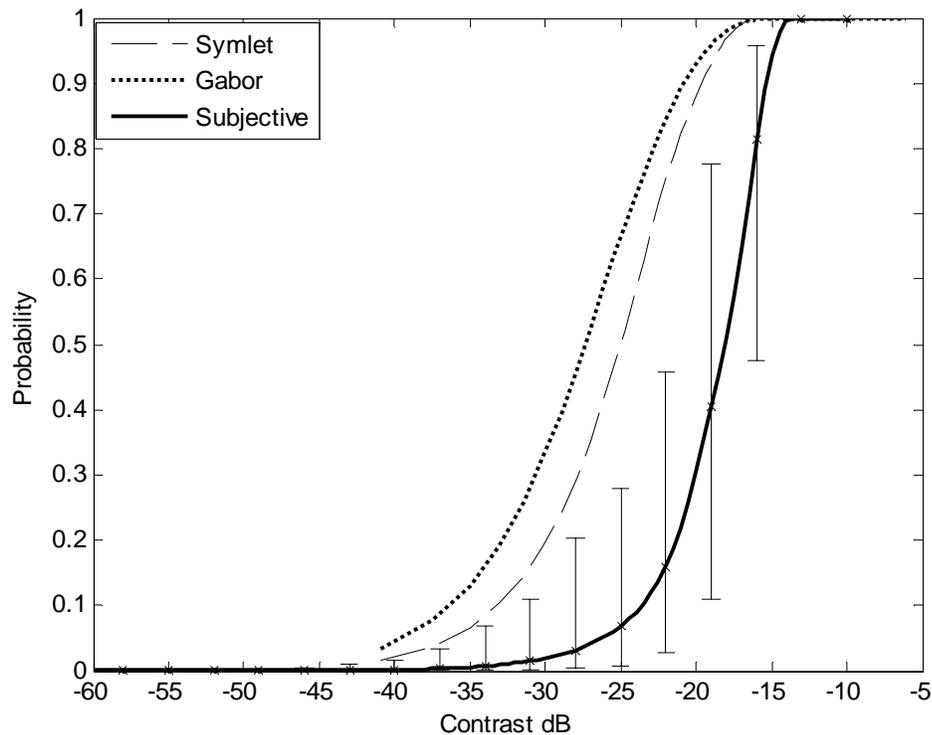
Figure 4.1 Banding 1-1 using bootstrapping mean, low frequency small envelope banding pattern. Assumption is made that HVS detects only the absolute maxima when observing a defect pattern.
