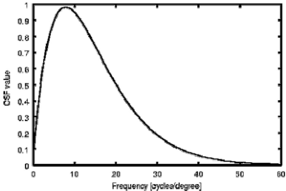
Figure 1.1 Contrast Sensitivity curve as a function of frequency adapted from [7]
