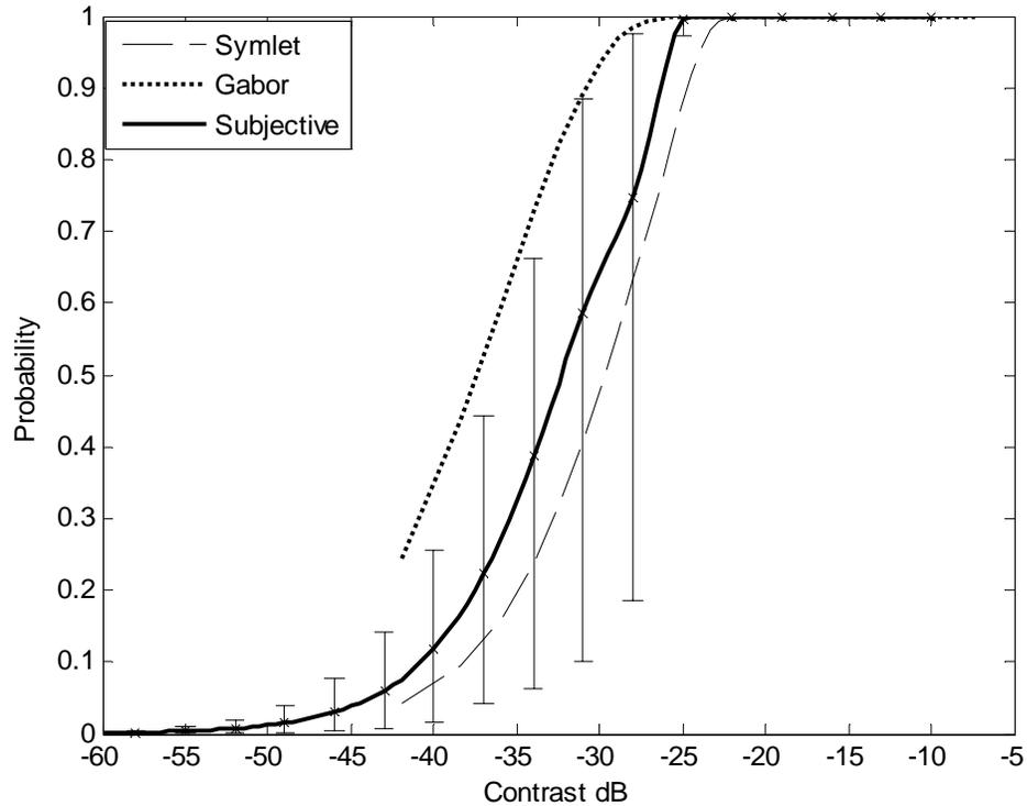
Figure 4.2 Banding 1-2 using bootstrapping mean, low frequency, large envelope banding pattern. Assumption is made that HVS detects only the absolute maxima when observing a defect pattern
