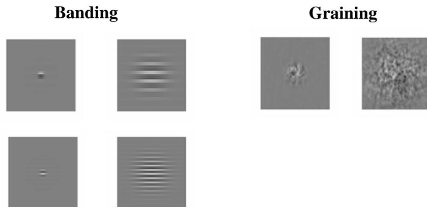
Figure 3.2 Banding and Graining Defect Patterns
