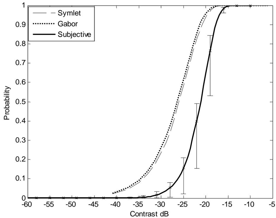
Figure 4.5 Banding 1-1 using bootstrapping median, low frequency, small envelope banding pattern. Assumption is made that HVS detects only the absolute maxima when observing a defect pattern.
