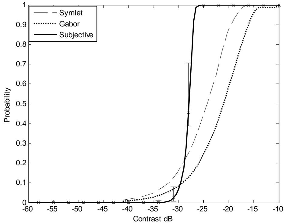
Figure 4.8 Banding 2-2 using bootstrapping median, high frequency, large envelope banding pattern. Assumption is made that HVS detects only the absolute maxima when observing a defect pattern.
