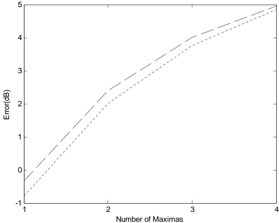
Figure 4.10 Number of maximas vs. Performance Error between Symlets prediction and Subjective results and Gabor prediction and Subjective results for the case of median. The smallest error occurs at one maximas for Symlet and one for Gabor prediction.
