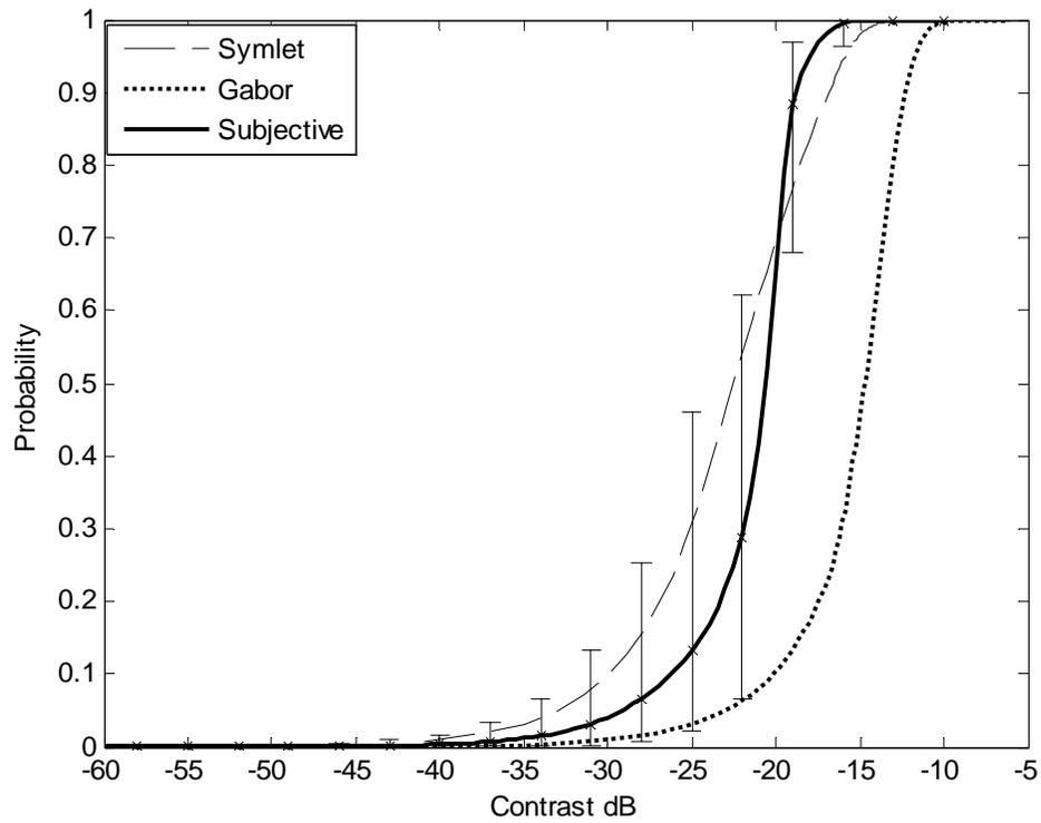
Figure 4.3 Banding 2-1 using bootstrapping mean, high frequency, small envelope banding pattern. Assumption is made that HVS detects only the absolute maxima when observing a defect pattern
