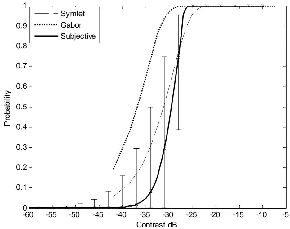
Figure 4.6 Banding 1-2 using bootstrapping median, low frequency, large envelope banding pattern. Assumption is made that HVS detects only the absolute maxima when observing a defect pattern.
