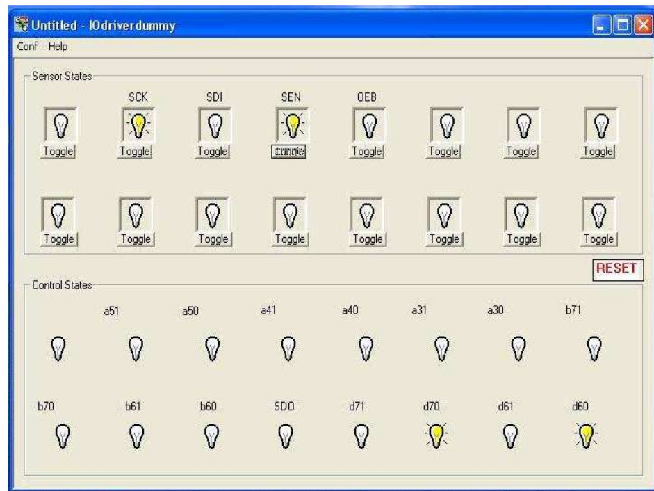
Figure 6.9: An example simulator of scanner control unit in register write back mode
