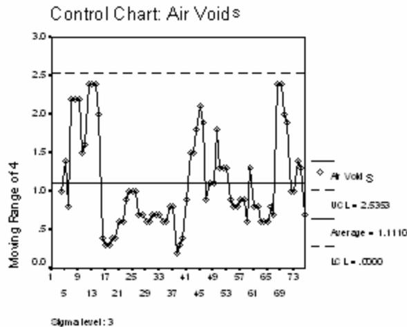
Figure 4.5 Moving Average Control Chart for HMA Air Voids: Moving Range
