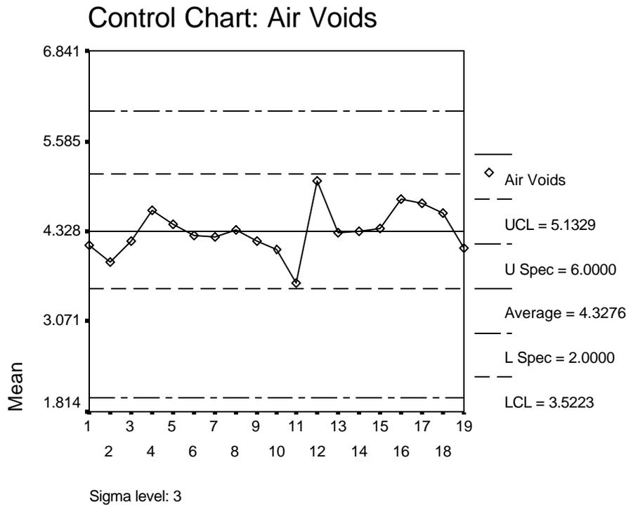
Figure 4.2 Establishing an  $\bar{x}$ -Chart for HMA Air Voids
