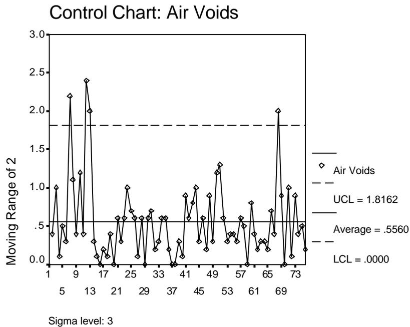
Figure 4.3 Individual Control Chart for HMA Air Voids: Moving Range
