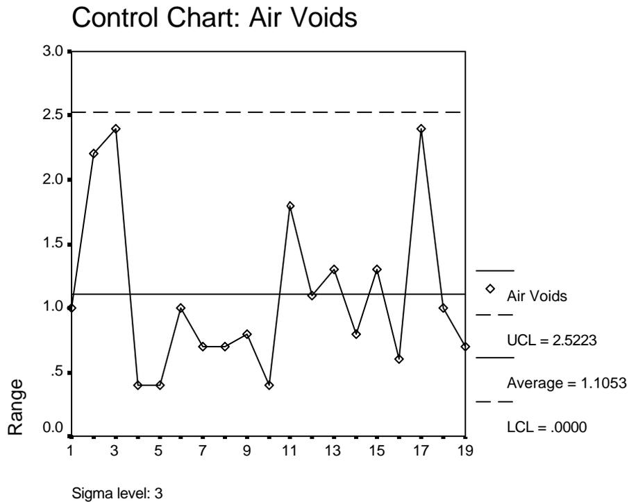
Figure 4.1 Establishing R-Chart for HMA Air Voids
