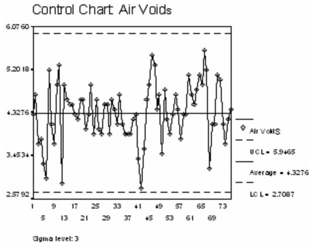
Figure 4.4 Individual Control Chart for HMA Air Voids: Individual Observations
