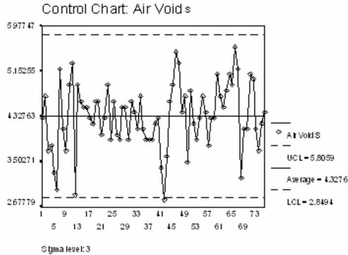
Figure 4.6 Moving Average Control Chart for HMA Air Voids: Moving Average
