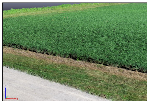
Figure 5. A side view of the alfalfa canopy in Field 1 from a portion of a fully processed model flown on 4 June 2019 using 30–90° flight parameters. Although the UAV did not take pictures from this angle and this close to the ground, the photogrammetry process captured the transition from the short grass bordering the field to the taller alfalfa plants.
