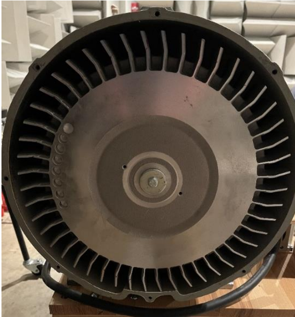
Figure 3-7 The 48-blade rotor of the regenerative blower used on the muffler test rig.
