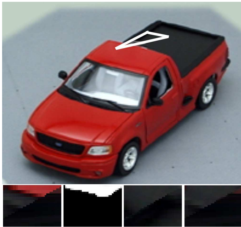
Figure 3.5: (Top) Exemplar image from the "truck" data set. Triangle outlined in white on cab illustrates a partially occluded surface facet from this view. (Far left) Partially occluded facet extracted and warped. (Middle left) Pixels determined to be occluded shown in white. (Middle right) Closest neighbor facet that contains visible pixels. (Far right) Synthesized facet containing only visible data.
