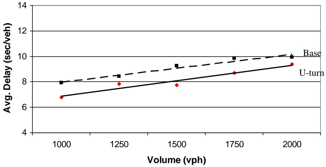
Figure B-1. Average delays, 5 percent left turns and 15 percent U-turns
