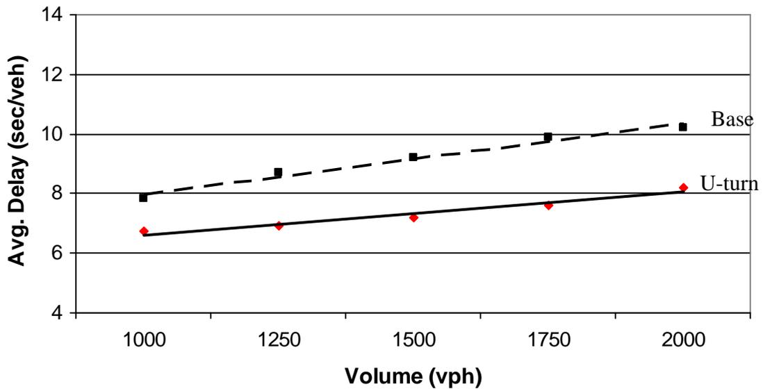
Figure B-2. Average delays, 5 percent left turns and 20 percent U-turns
