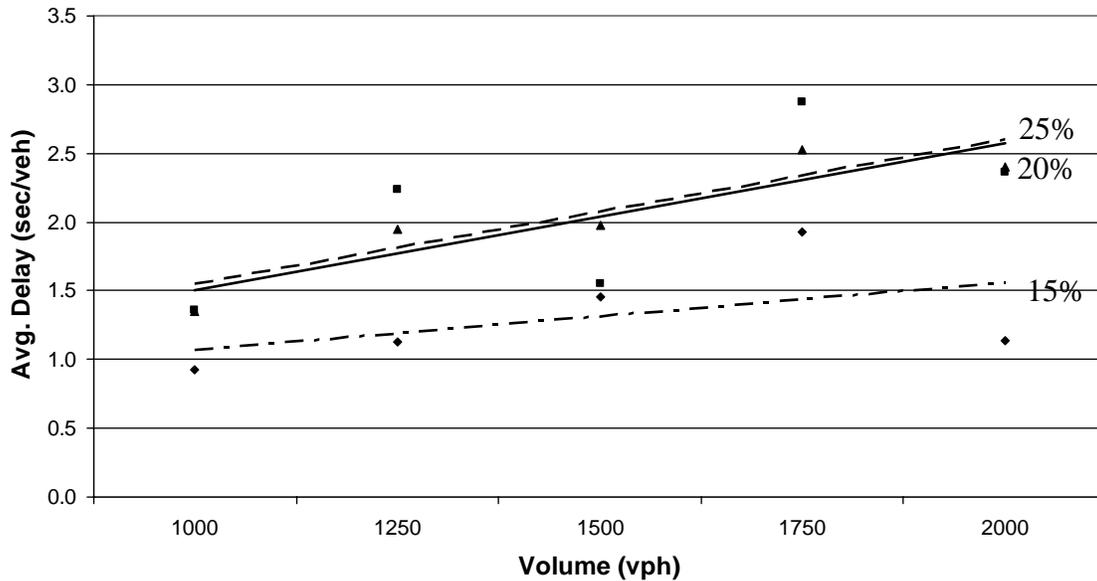
**Figure 6. Delay differences between Base and U-turn scenarios, 10 percent left turns**
