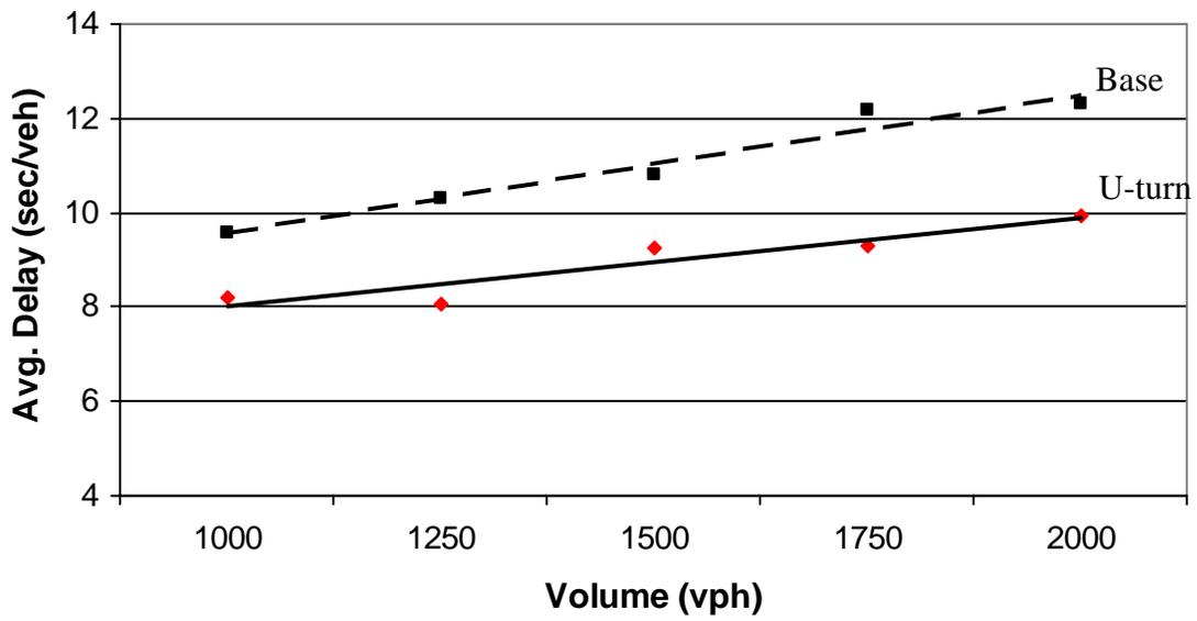
Figure B-5. Average delays, 10 percent left turns and 20 percent U-turns
