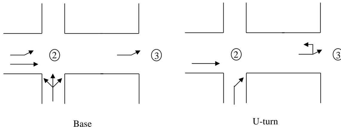
**Figure 3. Movements for weighted average delay estimates**
