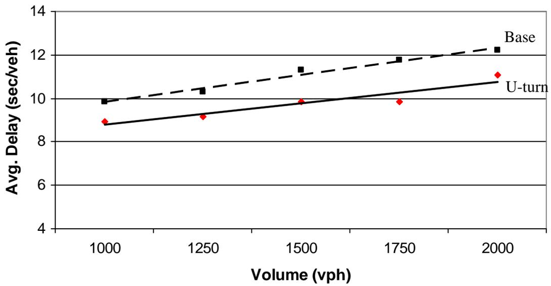
Figure B-4. Average delays, 10 percent left turns and 15 percent U-turns
