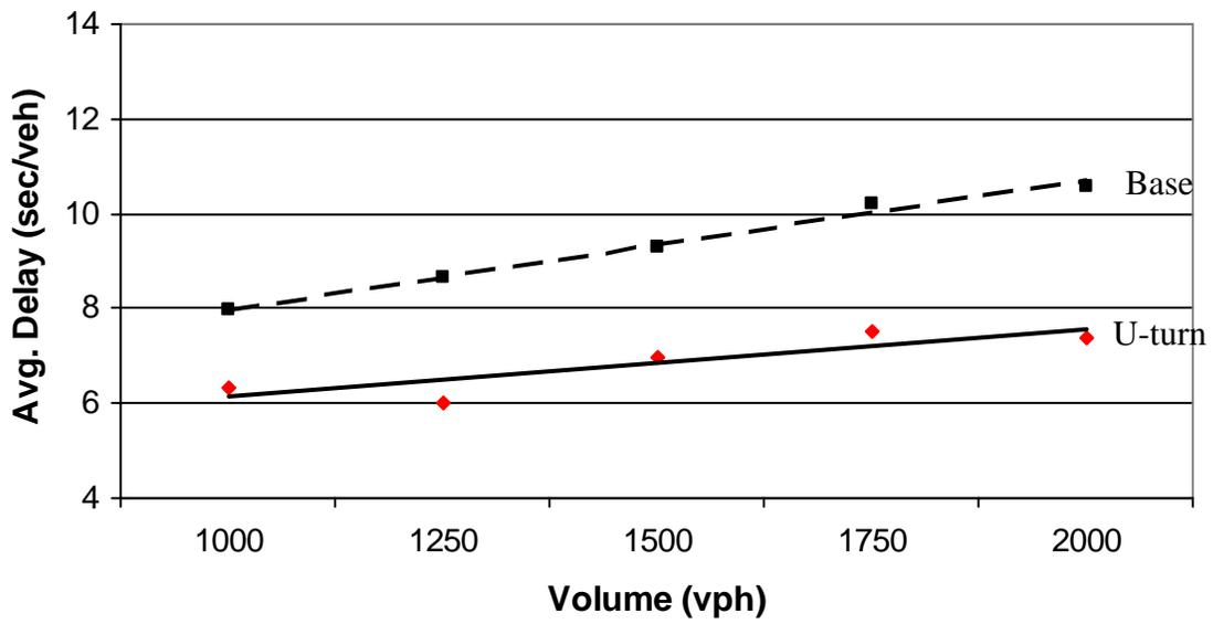
Figure B-3. Average delays, 5 percent left turns and 25 percent U-turns
