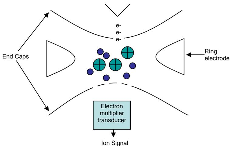
Figure 1.4. Quadrupole ion trap operation.
