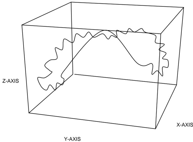
Figure 1.8 Lissajous curve of ion motion.
