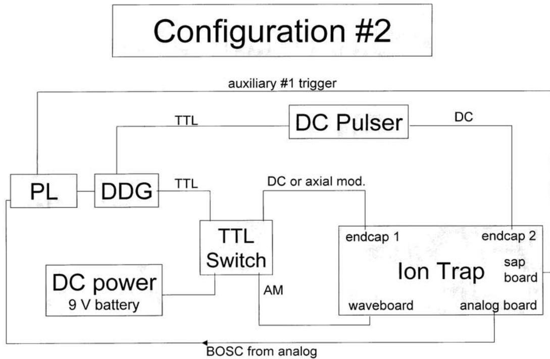
Figure 2.5. Circuit diagram for DC tomography experiment.
