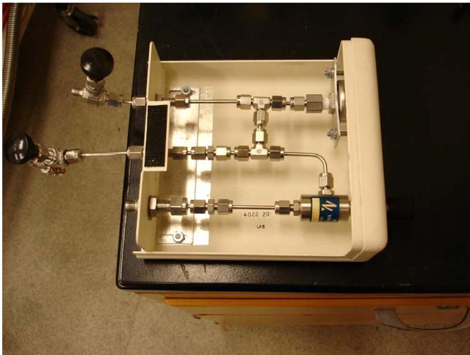
Figure 2.6. FinniganMAT vacuum delivery system.
