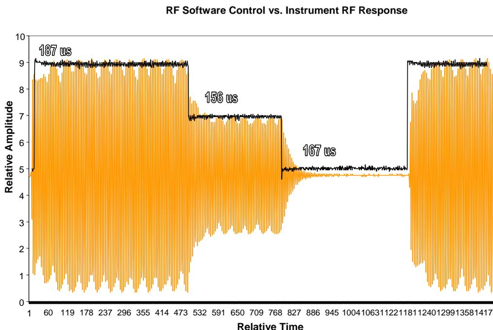
Figure 3.1. Shows the relative lag time between the software control settings of the RF level and the actual instrumental response.
