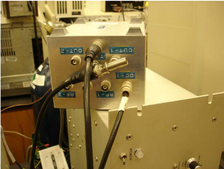
Figure 2.4. TTL switch box.
