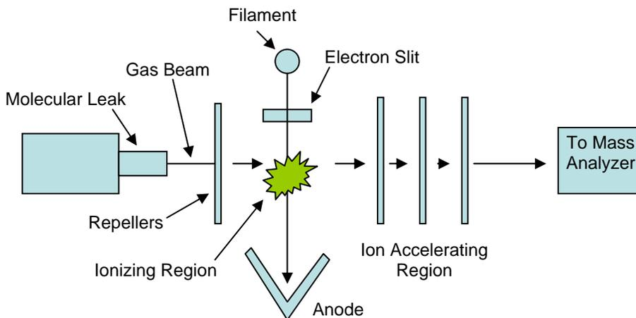
Figure 1.3. Electron impact ionization source.
