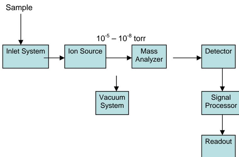
Figure 1.2. Components of a Mass Spectrometer.
