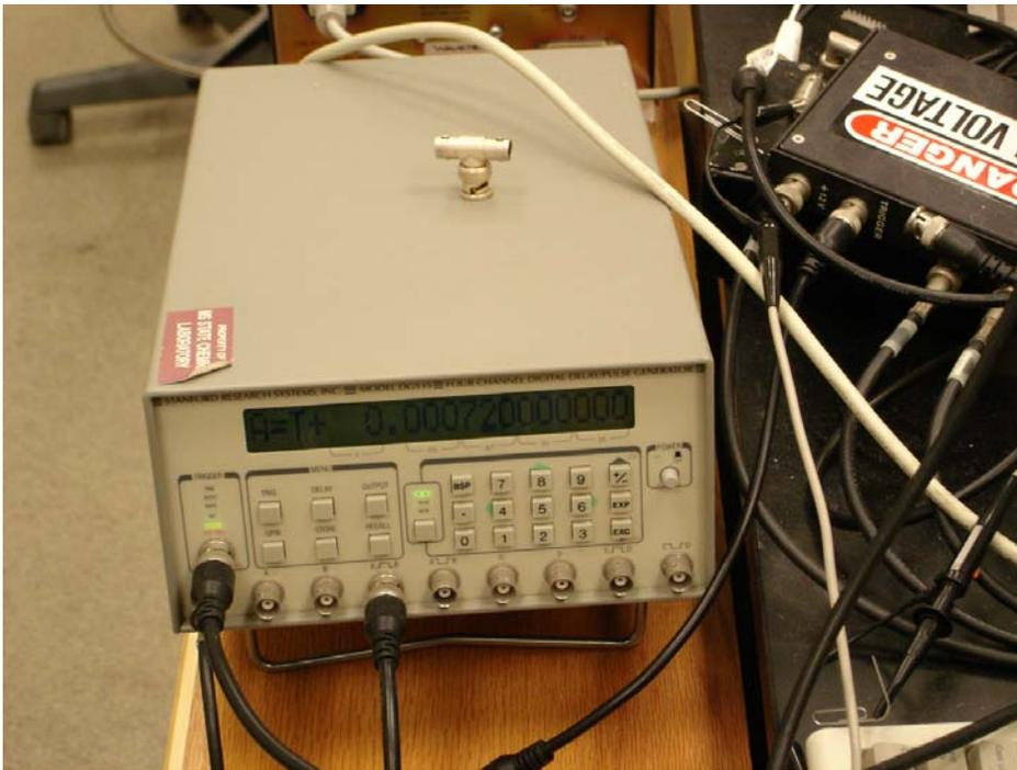
Figure 2.3. Digital delay generator.
