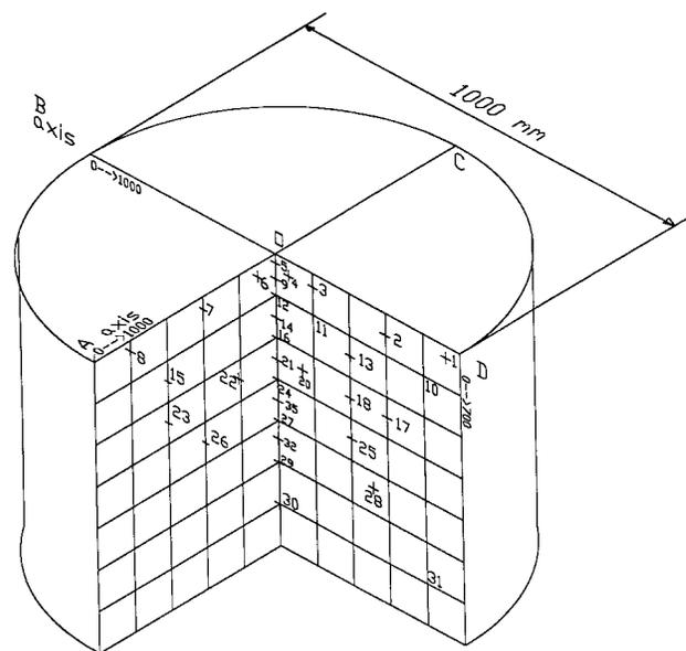
**Figure 1—Thermocouple location map for Tests 1, 2, and 3 of NI treatment. Grid is on 100-mm interval.**
