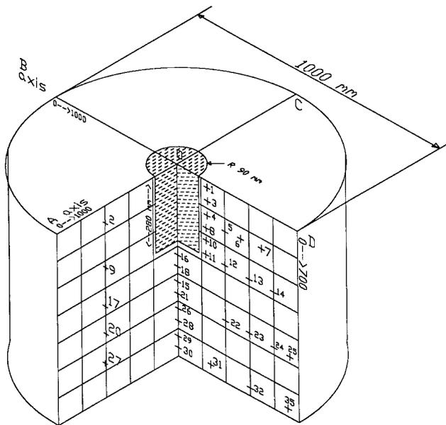
Figure 2—Thermocouple location map for Tests 4, 5, and 6 of STI treatment. Grid is on 100-mm interval.
