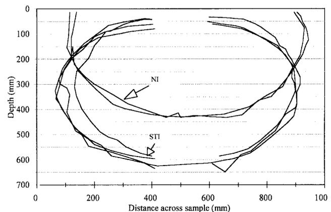
Figure 6—Water penetration depth versus distance across the sample along A and B axes for NI (test 3) and STI (tests 5 and 6) treatments.
