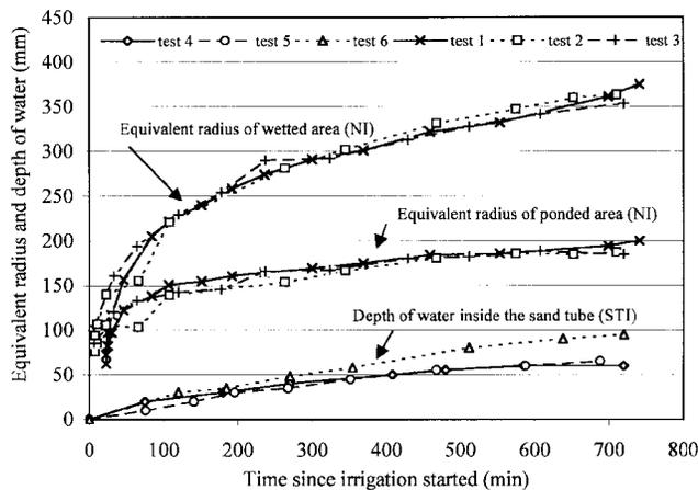
Figure 3—Depth of water rise inside the sand tube during irrigation, STI treatment, and equivalent radius of the ponded surface and the wetted area, NI treatment, is plotted vs time since irrigation started. Depth of sand tube was 280 mm.
