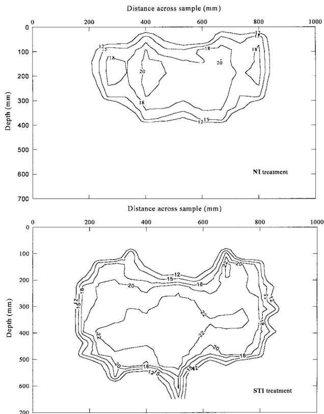
Figure 7—Contour plot of moisture content (%) distribution for NI and STI treatments.
