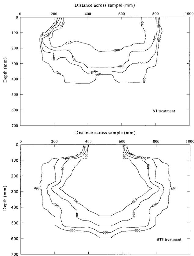
Figure 5—Wetting front position (isolines are time in min), during NI and STI treatment.
