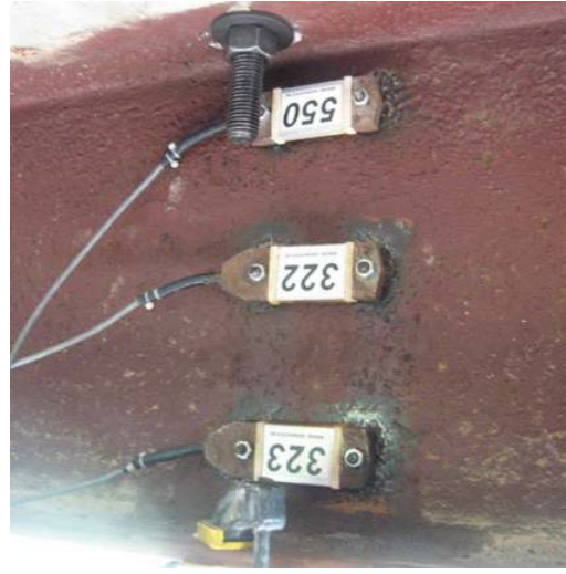
(b) Attached reusable strain gages
