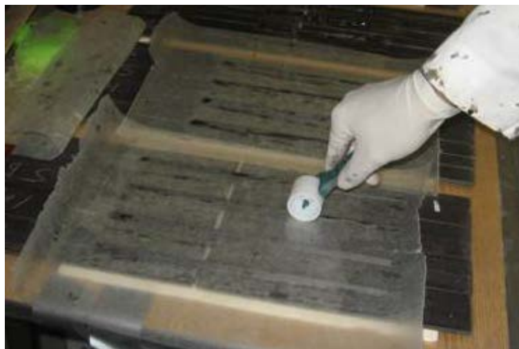
(b) Pressing on to steel surface with roller
