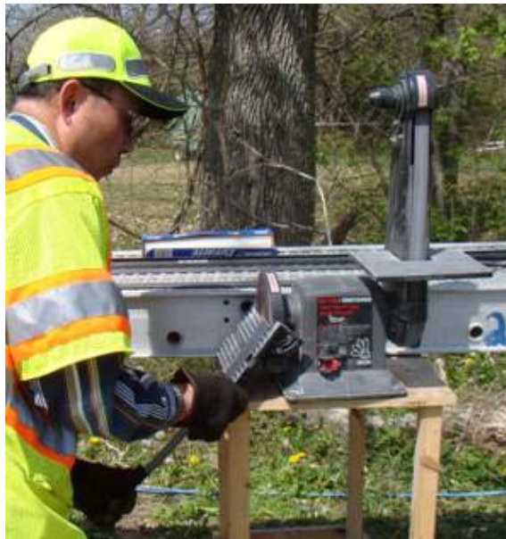
Fig. 5.16: Sanding laminate edges to obtain reverse taper
