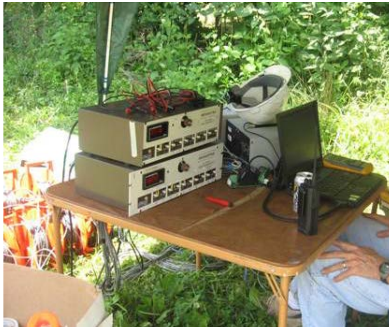
Fig. 5.27: Data acquisition to laptop computer via two signal conditioners
