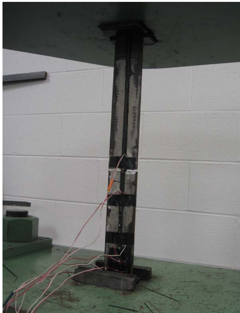
Fig. 2.9: Tensile testing of double strap joint specimen
