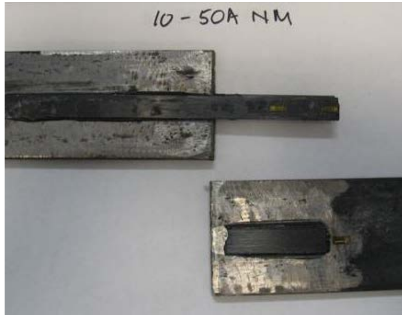
Fig. 2.12: Typical CFRP delamination seen in normal modulus CFRP
