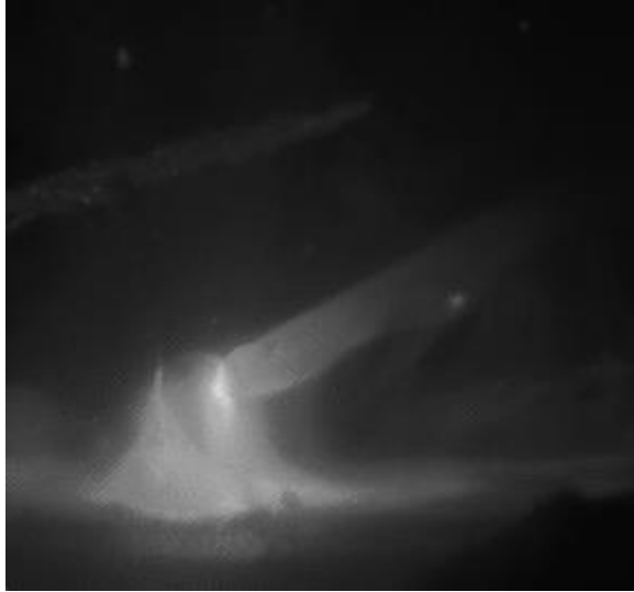
Figure 6.17 Examples of the mixed mode in DE-GMAW.
