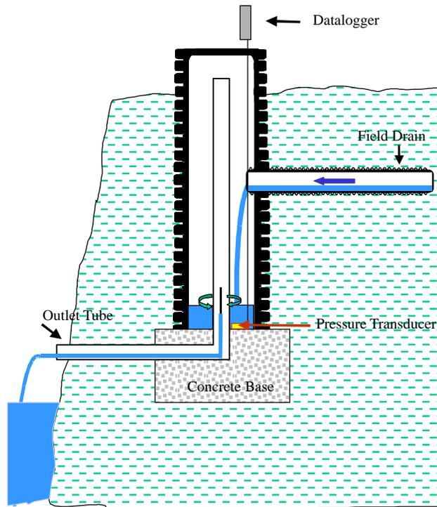
**Figure 1.** Schematic of the flow monitoring system. Flow enters the system through the field drain. Water is contained in the vertical riser, exits through the slotted weir, and is discharged into the outlet tube. Some dimensions are exaggerated to indicate the process.
