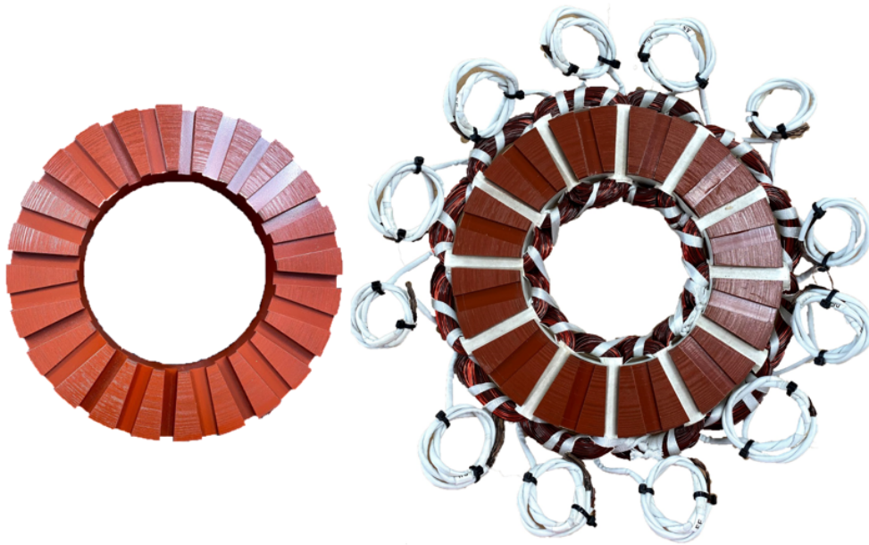
Figure 3.35: The prototyped profiled stator core and active stator wound with coils.
