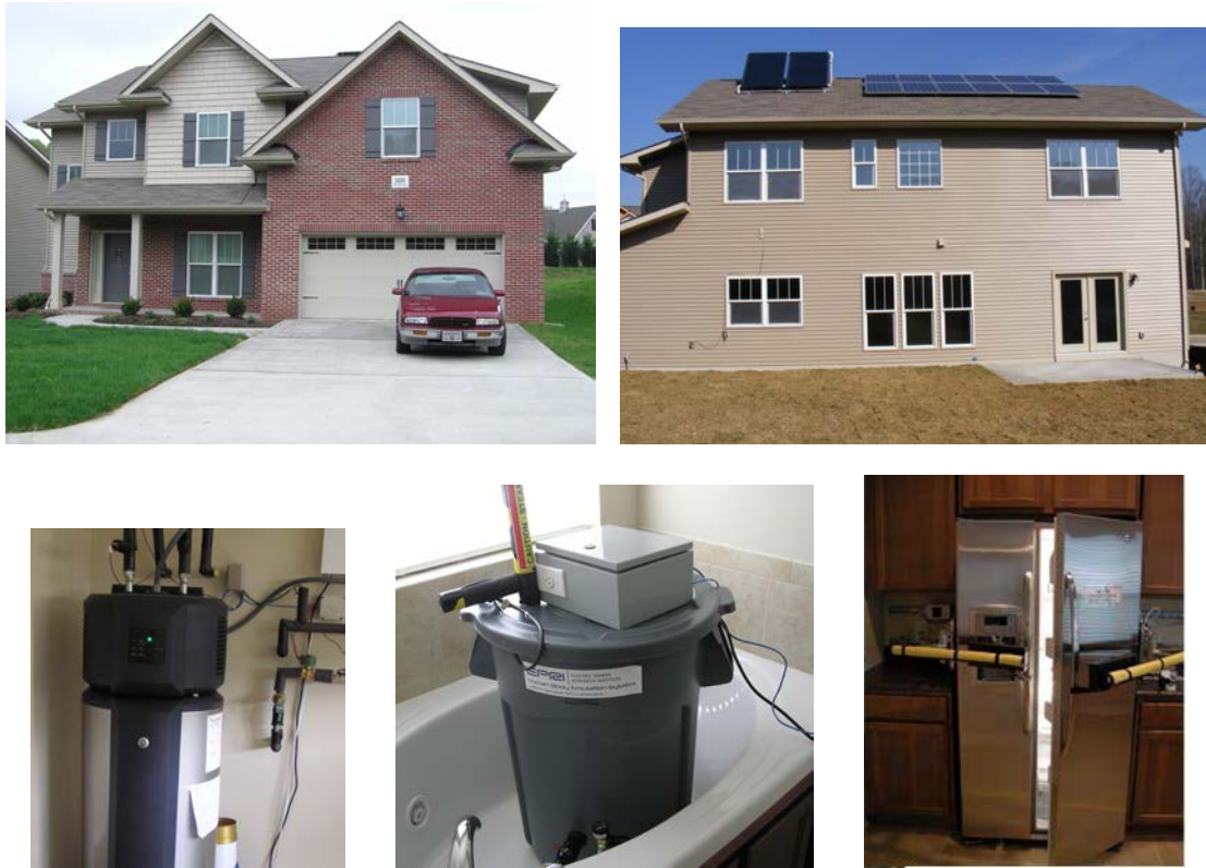
Figure 4.3: The near net-zero-energy (NNZE) house front (a) and back (b). TVA robotic devices are controlled to mimic realistic human behavior. Also shown is a HPWH used in the retrofit house (c), a shower emulator (d), and a refrigerator with programmed arms (e) that operate according to automatic schedules.
