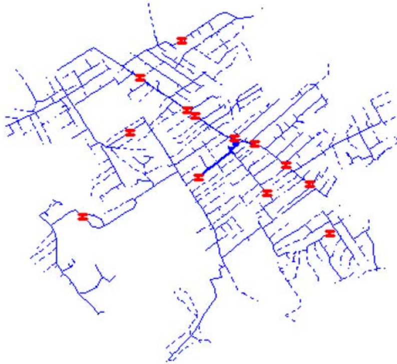
Figure 2.5: Circuit schematic of LGEs1, indicating the location of its 13 CBs.
