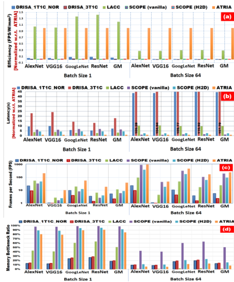
Figure 5.6: (a) Efficiency (FPS/W/mm 2 ), (b) latency, (c) throughput (FPS), and (d) memory bottleneck ratio (MBR) results for various in-DRAM accelerators across CNNs. GM means geometric mean.
