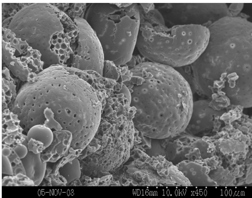
Figure 9: Fractured microspheres prepared from a double emulsion technique
