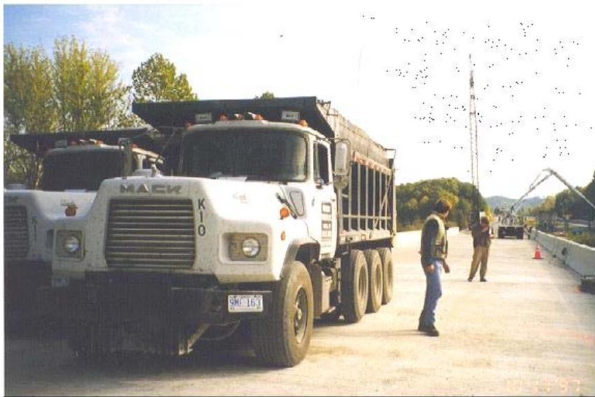
**Figure 13.** Test Vehicles – Tandem Axle Trucks (Third Rear Axle not Engaged).
